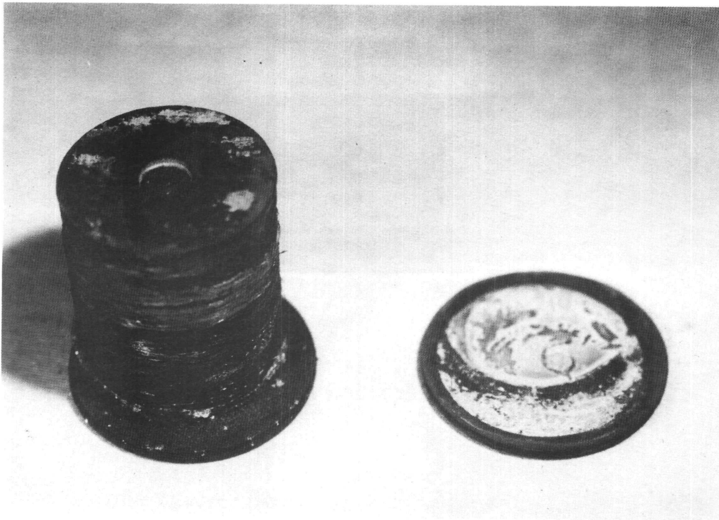
Figure 18. Isothermal Weight Loss Leg No. 6 900°C i1/A=8
