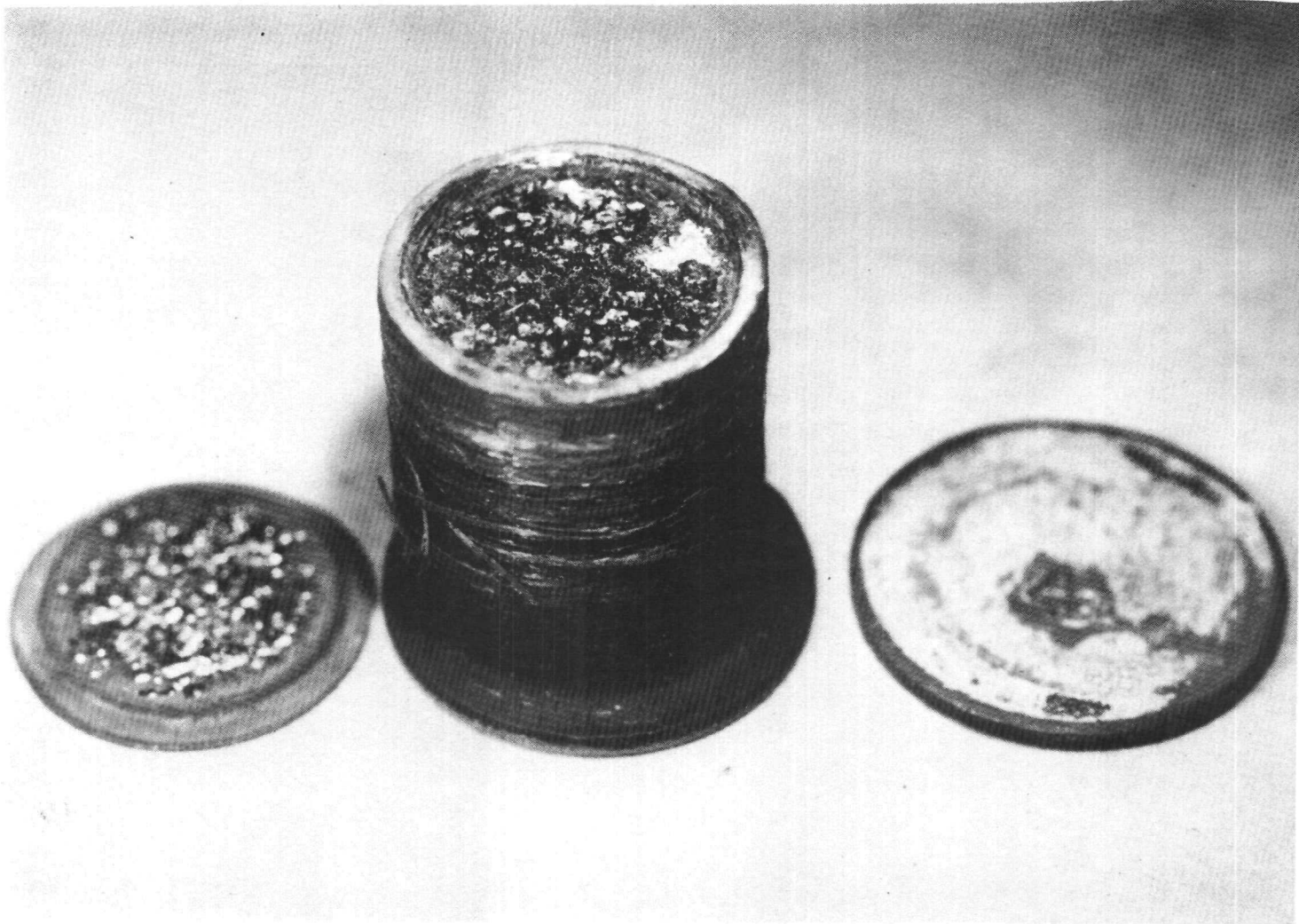
Figure 16. Isothermal Weight Loss Leg No. 4 850°C il/A=8
