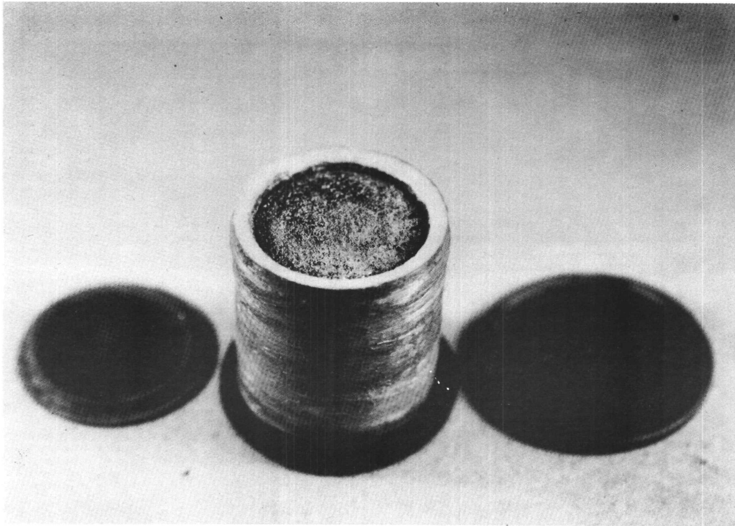
Figure 14. Isothermal Weight Loss Leg No. 2 800°C il/A=8
