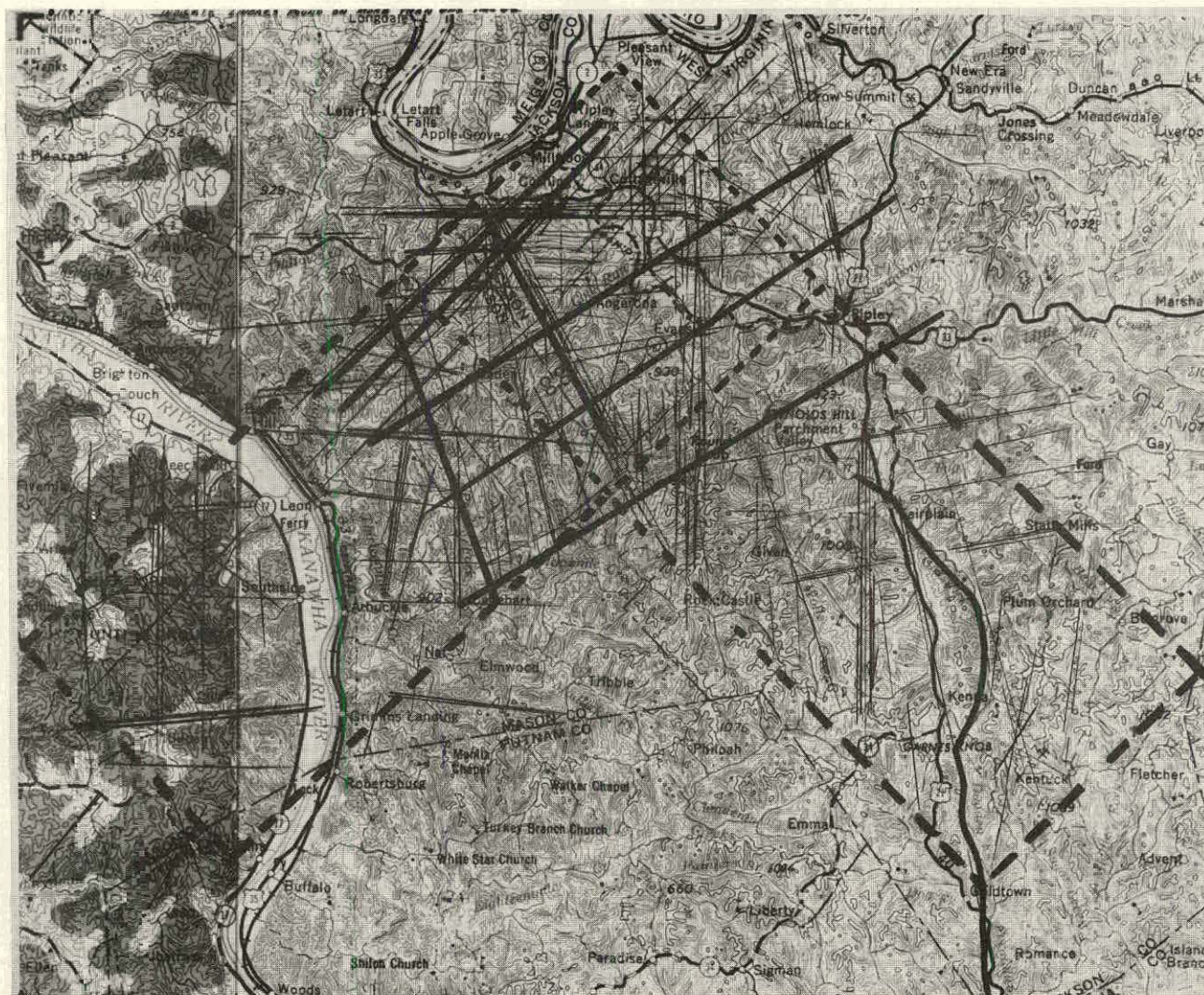
FIGURE 5. VISUALLY INTERPRETED LINEAMENTS IN THE COTTAGEVILLE AREA. Thick Lines are More Prominent and Definite, Thin Lines are More Tenuous.
