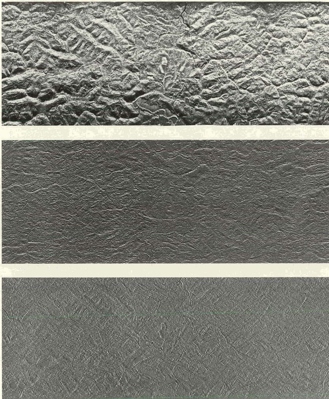
FIGURE 2. GRADIENT FILTERING OF A SYNTHETIC APERTURE RADAR IMAGE OF COTTAGEVILLE, WEST VIRGINIA AREA. (a) Unfiltered Image. (b) Image filtered in NE-SW Direction, +45^{\circ} Passband. (c) Image filtered in NW-SE direction, +45^{\circ} passband.
