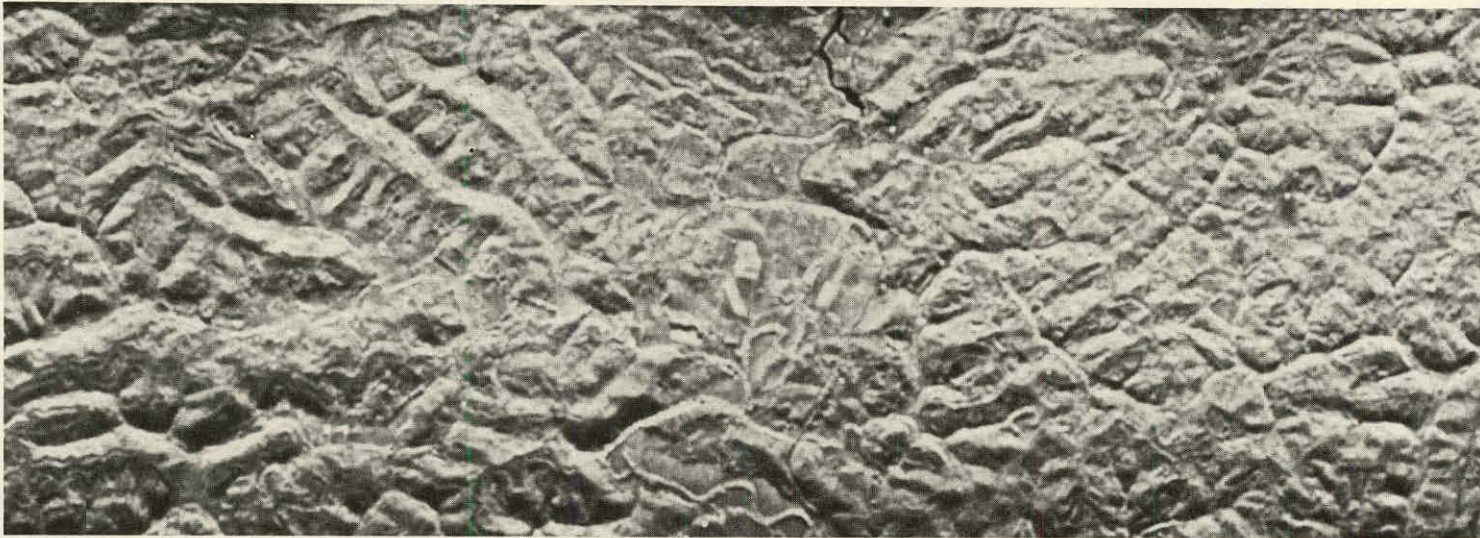
FIGURE 11. LOW-PASS FILTERING OF SAR IMAGERY ( \lambda=3\text{cm} ) OF COTTAGEVILLE FIELD. 9\times 9 Smoothing.
