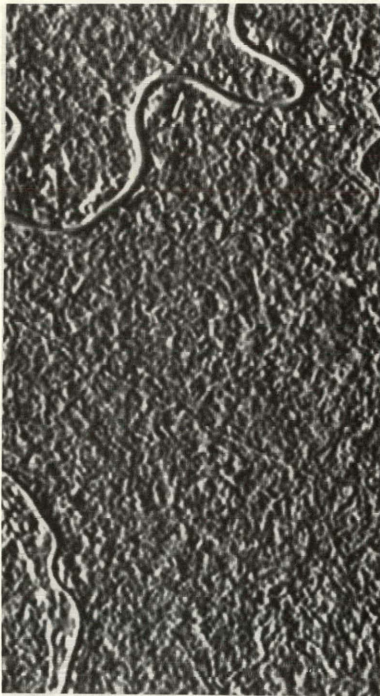
FIGURE 16. SHADED RELIEF "MAP" OF LANDSAT IMAGERY OF COTTAGEVILLE WITH SIMULATED SUN 30^{\circ} ABOVE HORIZON IN THE EAST DIRECTION.
