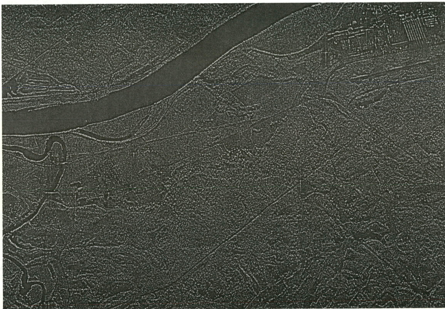
FIGURE 10. HIGH-PASS FILTERING OF PORTION OF SAR IMAGERY ( \lambda=3\text{cm} ) OF COTTAGEVILLE REGION. Note Enhancement of Cultural Features, Particularly the Large Industrial Plant on the Ohio River.
