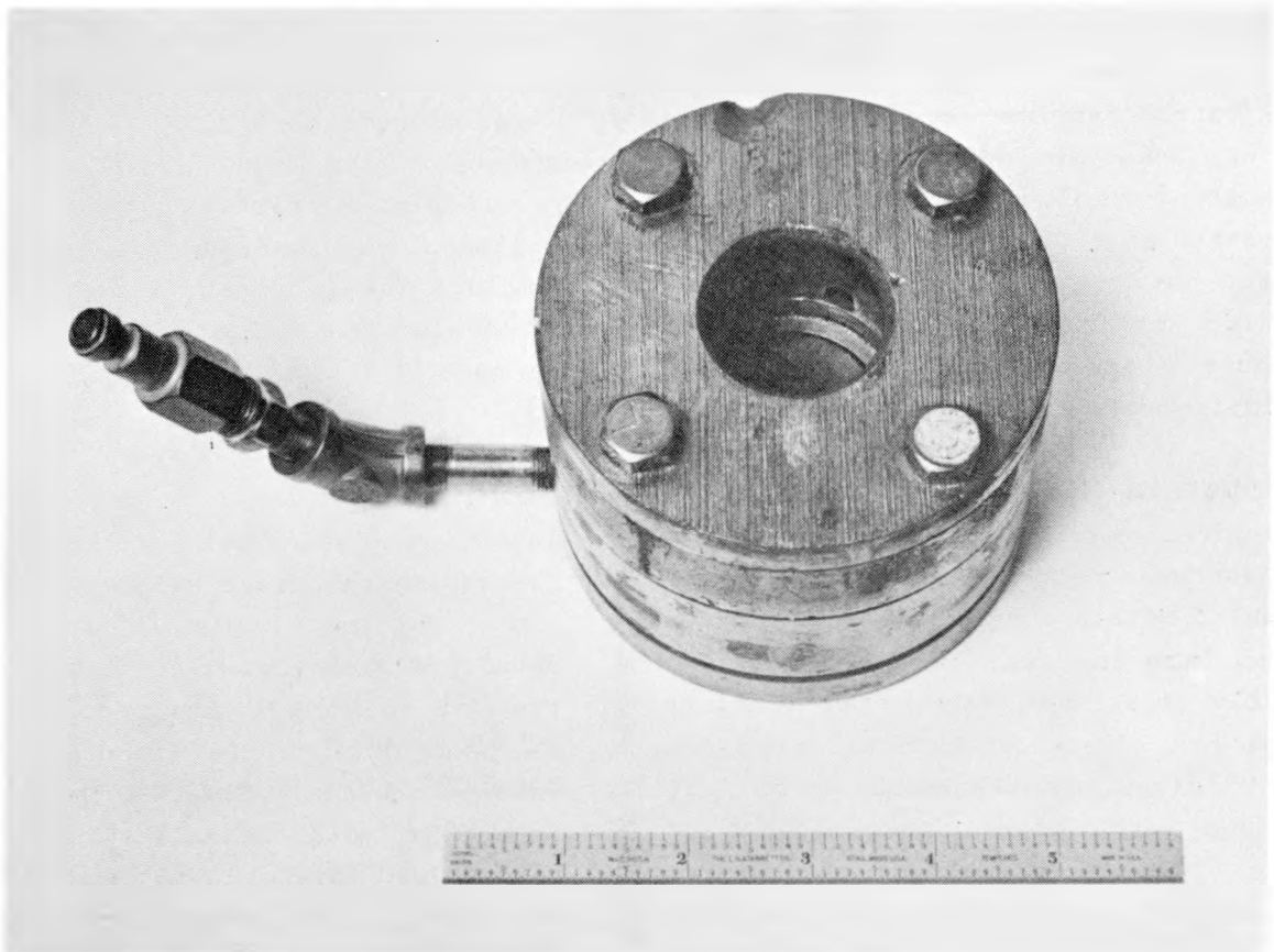
FIGURE 1 - Presently used mold consists of graphite and metal pieces.
