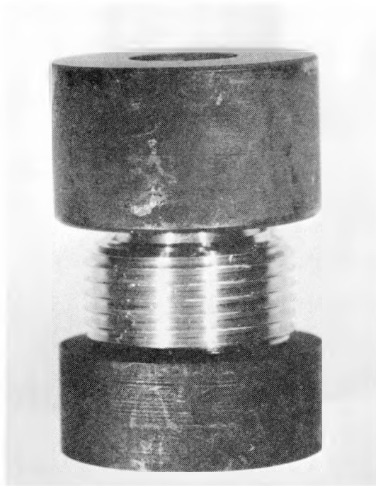
FIGURE 5 - Fixtured component ready for placement within the injection mold.
