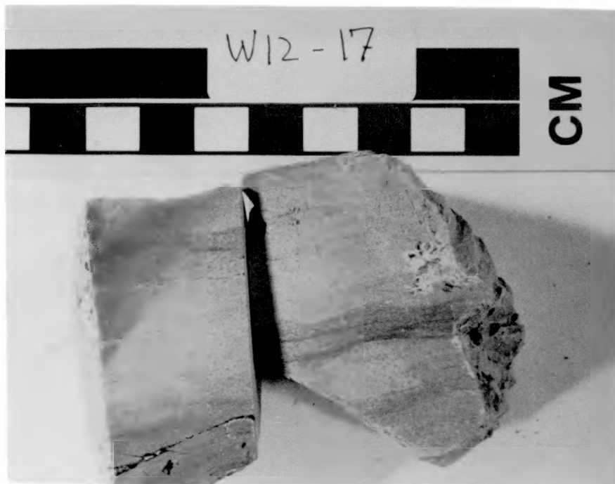
Figure VIII-14. Sample W12-17. Dolomite hand specimen with clay-rich layers.
