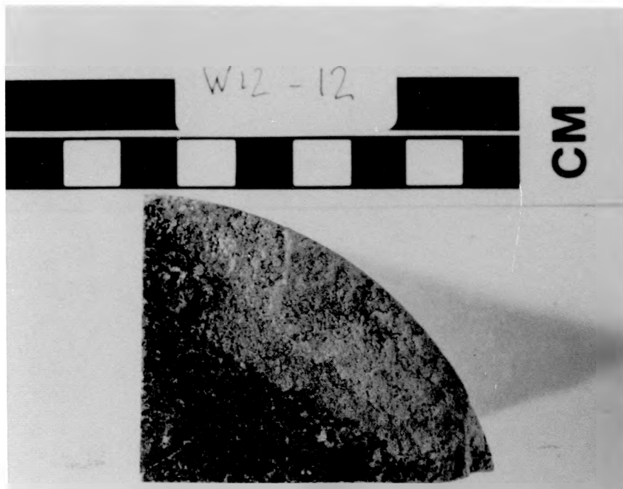
Figure VIII-36. Sample W12-12. Surface of open fracture in hand specimen.
