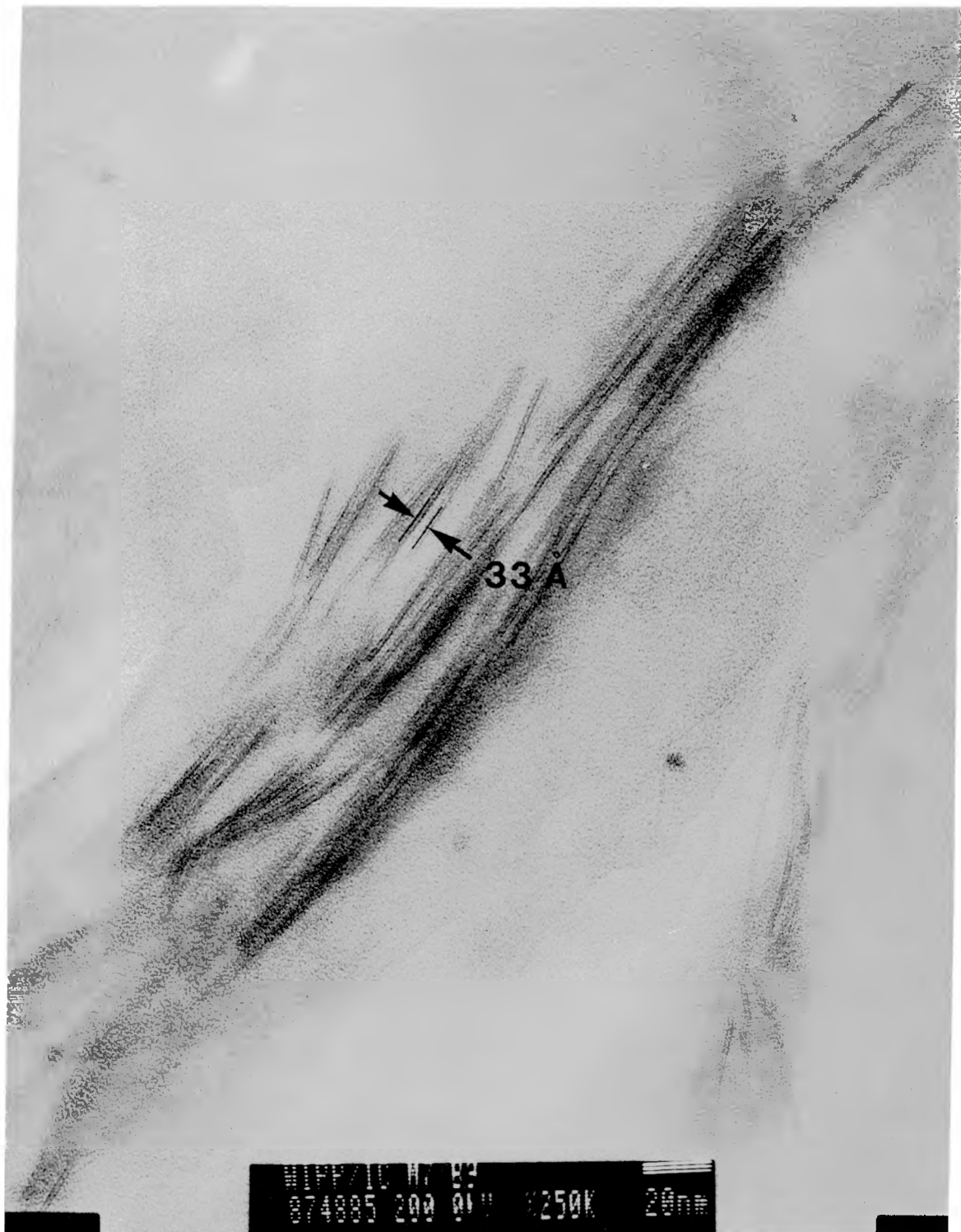
Figure VII-9. High-Resolution Lattice Fringe Image of Corrensite from Sample H6B-3.
