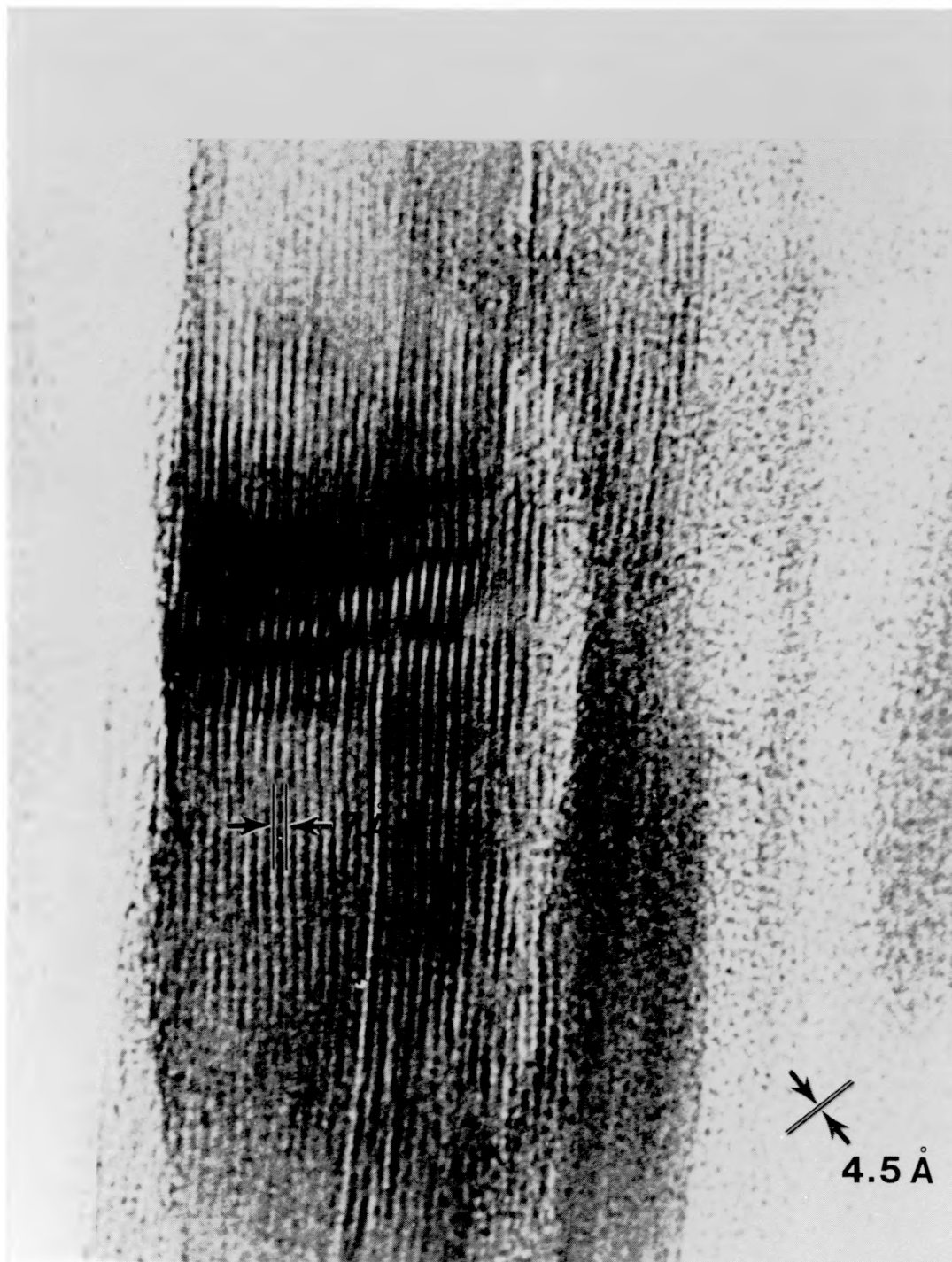
Figure VII-6. High-Resolution Lattice Fringe Image of Serpentine from Sample H6B-3.
