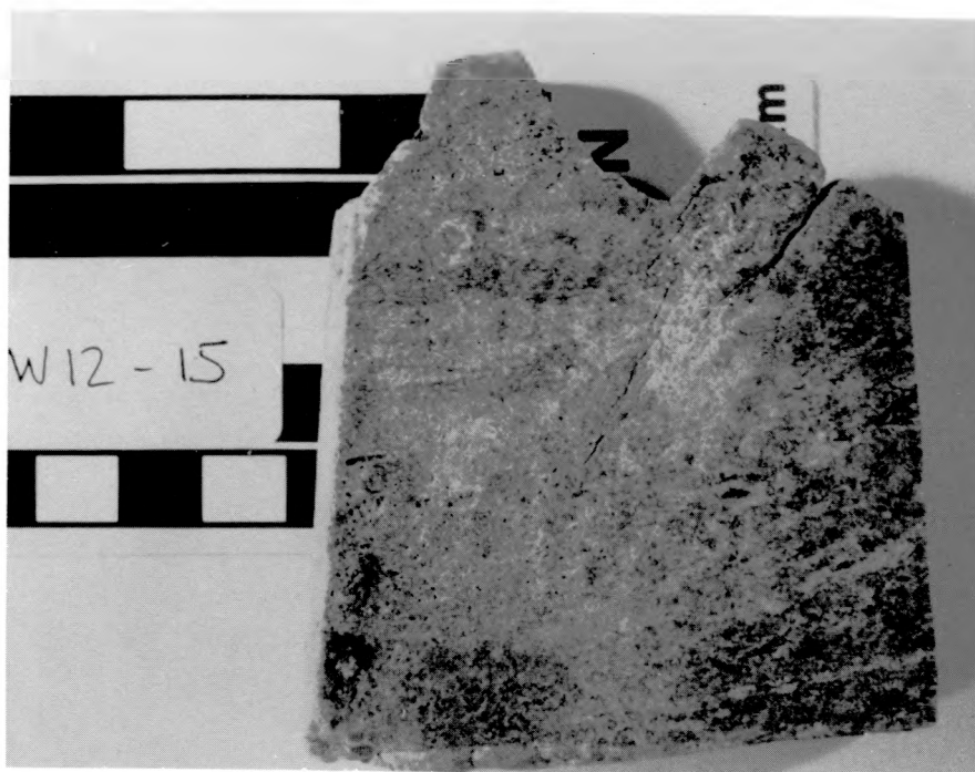
Figure VIII-30. Sample W12-15. Hand specimen showing various types of fractures.
