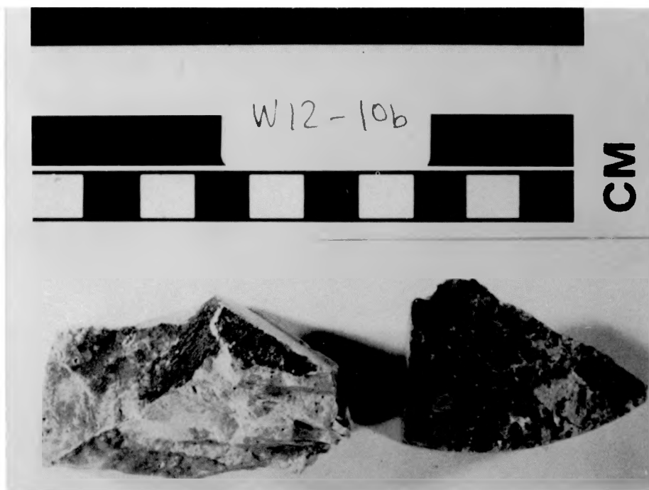
Figure VIII-37. Sample W12-10. Surface of open fracture in hand specimen.
