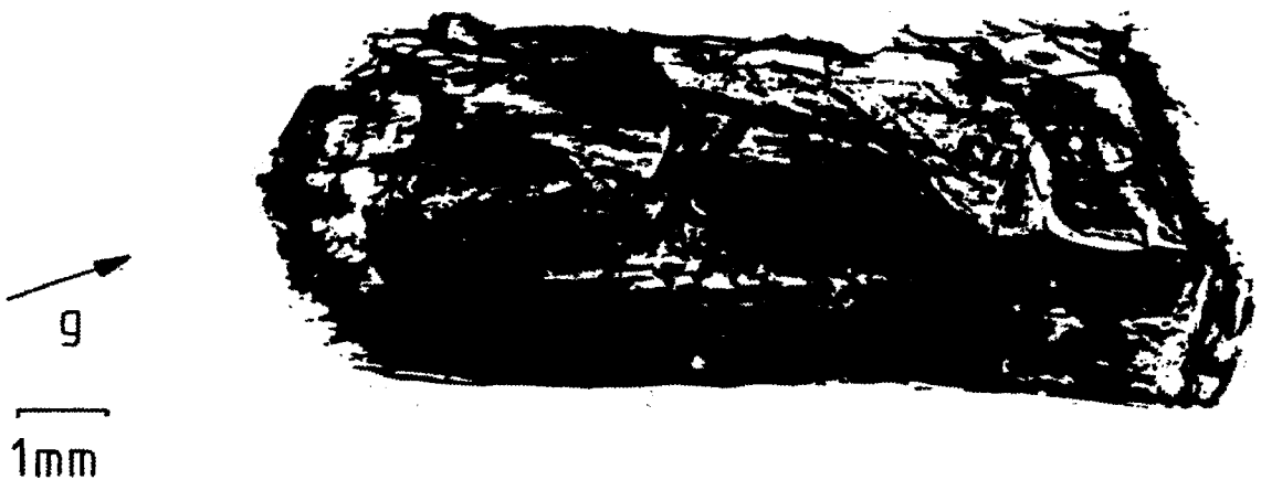
Figure 7. White Beam Synchrotron Topograph ( g = [112] , \lambda = 1\text{\AA} ), showing the detailed defect structure in the polymer crystal.
