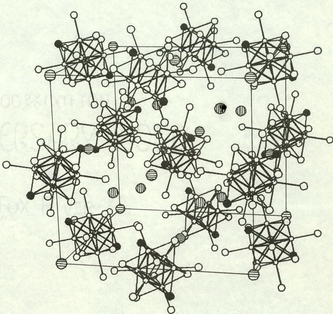
Figure 4. A perspective view of the  $(\text{Mo}_6\text{Cl}_7\text{S})\text{Cl}_6^{3-}$  clusters (darkened atoms lie on cluster's 3-fold axis) and chloride ions (crosshatched atoms) in the unit cell of  $(\text{C}_5\text{H}_5\text{NH})_3[(\text{Mo}_6\text{Cl}_7\text{S})\text{Cl}_6] \cdot 3(\text{C}_5\text{H}_5\text{NH})\text{Cl}$
