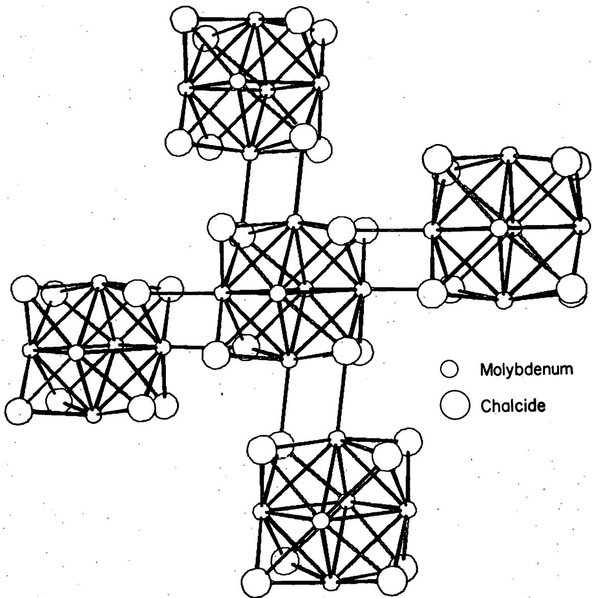
Figure 2. A perspective view of the arrangement of  $\text{Mo}_6\text{X}_8$  clusters in the Chevrel phases, with two of the six neighboring clusters deleted
