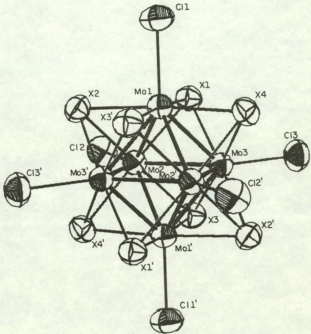
Figure 6. A labelled perspective view of the 50% probability thermal ellipsoids of the  $(\text{Mo}_6\text{Cl}_7\text{S})\text{Cl}_6^{3-}$  cluster
