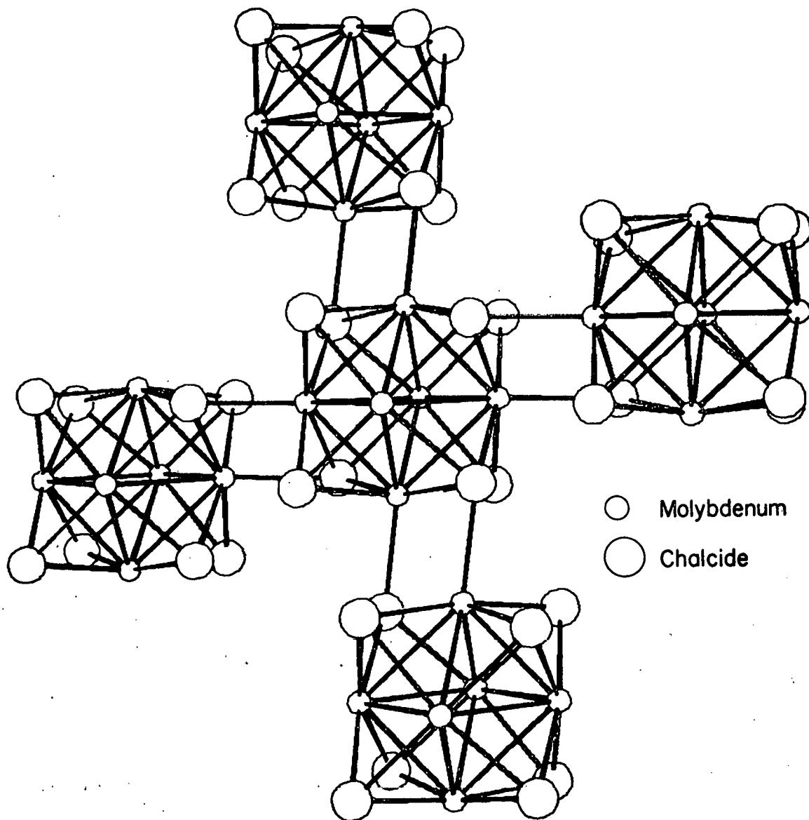
Figure 7. A perspective view of the arrangement of  $\text{Mo}_6\text{X}_8$  clusters in the Chevrel phases, with two of the six neighboring clusters deleted
