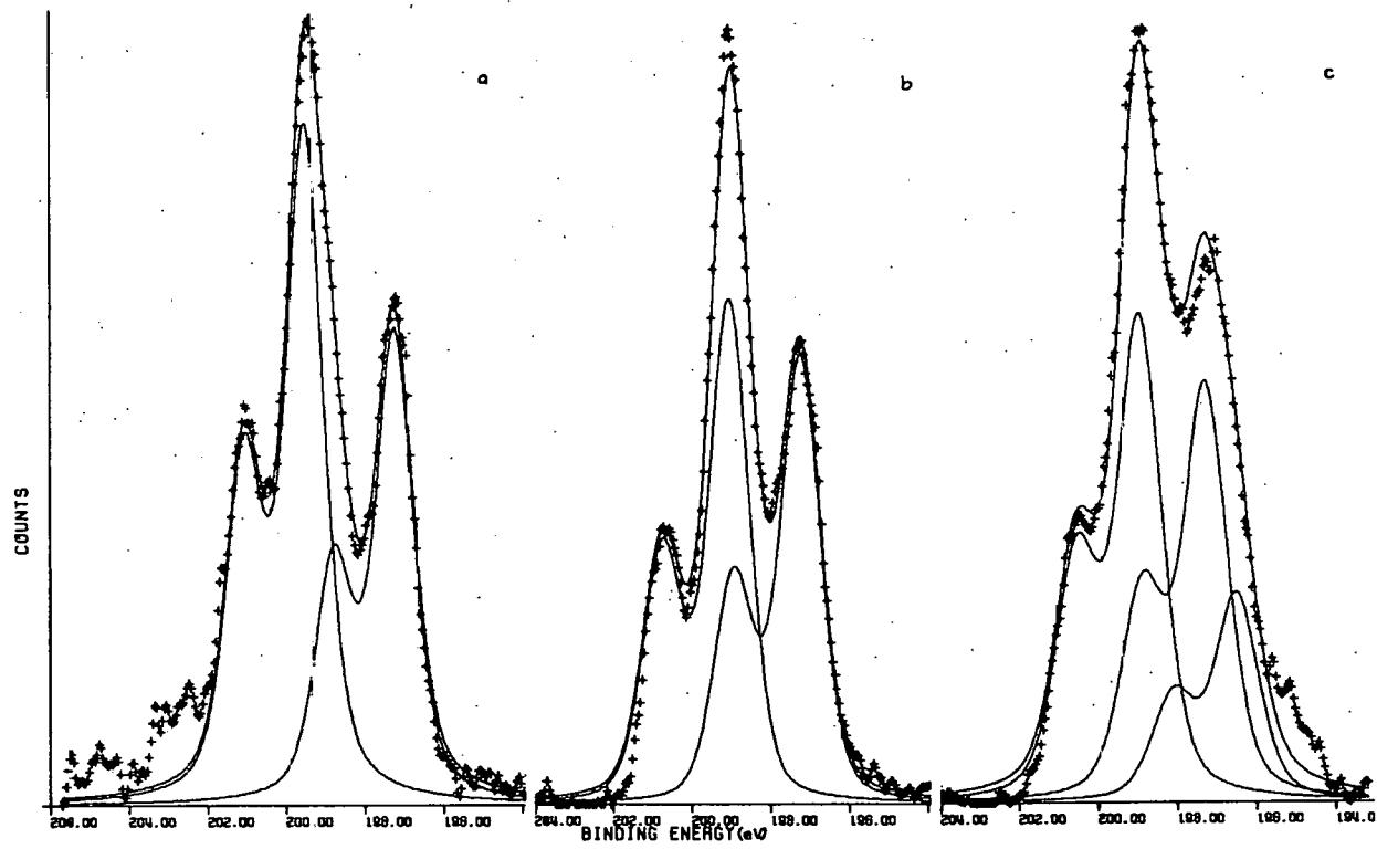
Figure 3. The chlorine 2p photoelectron spectra of  $[(n\text{-C}_4\text{H}_9)_4\text{N}]_2[(\text{Mo}_6\text{Cl}_8)\text{Cl}_6]$ , a;  $(\text{C}_5\text{H}_5\text{NH})_3[(\text{Mo}_6\text{Cl}_7\text{S})\text{Cl}_6]$ , b;  $(\text{C}_5\text{H}_5\text{NH})_3[(\text{Mo}_6\text{Cl}_7\text{S})\text{Cl}_6] \cdot 3(\text{C}_5\text{H}_5\text{NH})\text{Cl}$ , c
