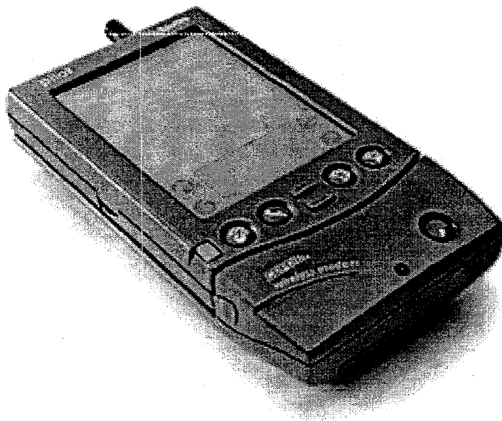
Fig. 3. Internet-ready handheld PalmPilot™ for remote data system access.
