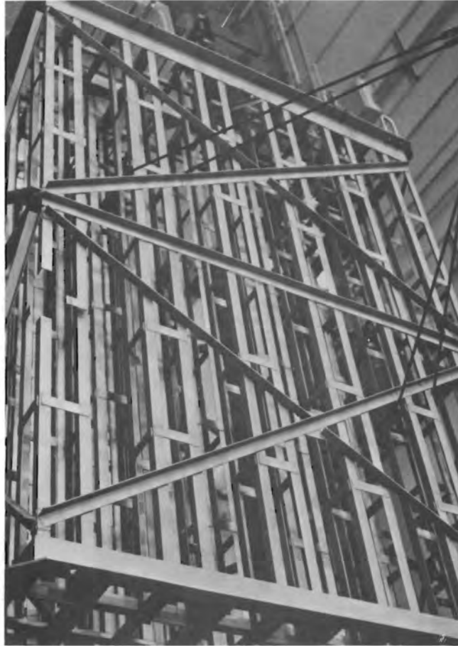
FIGURE 4A. 304 Stainless Steel Spent Fuel Pool Rack After 6-2/3 yr in Point Beach Reactor (PWR) Pool
