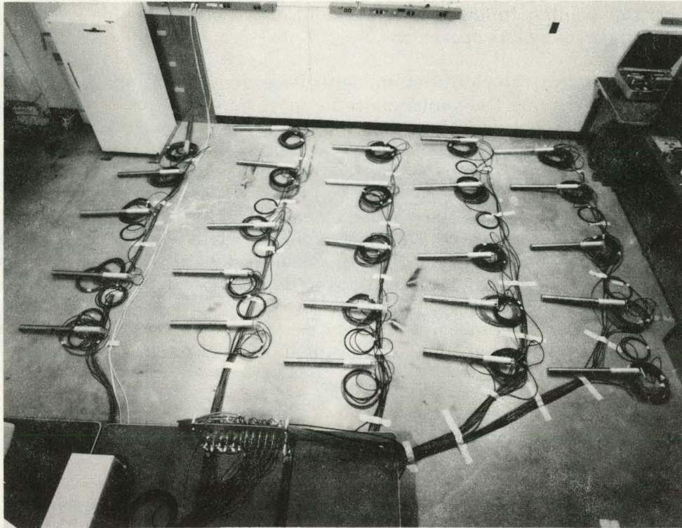
Fig. 6. Test configuration of the 25 neutron detectors at Los Alamos.
