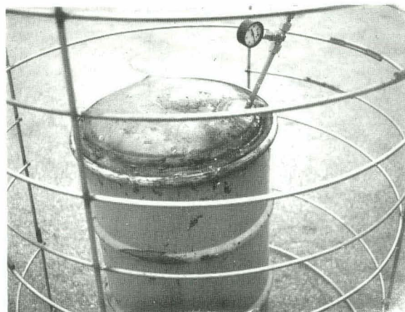
FIGURE 18 - Test setup with lid on secondary container.
