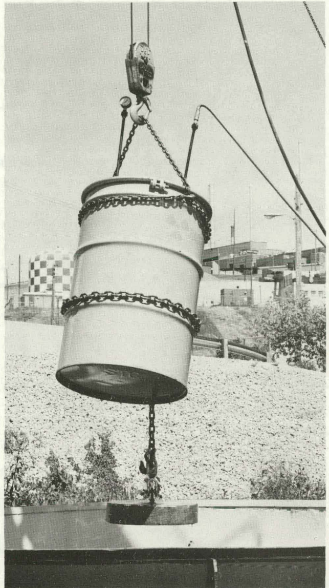
FIGURE 20 - Secondary container with weights added being lowered into water tank for test with compressed air.
