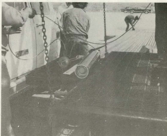
Figure 2 A-D. Close-up of Down Hole Television (DHTV) Camera Head
