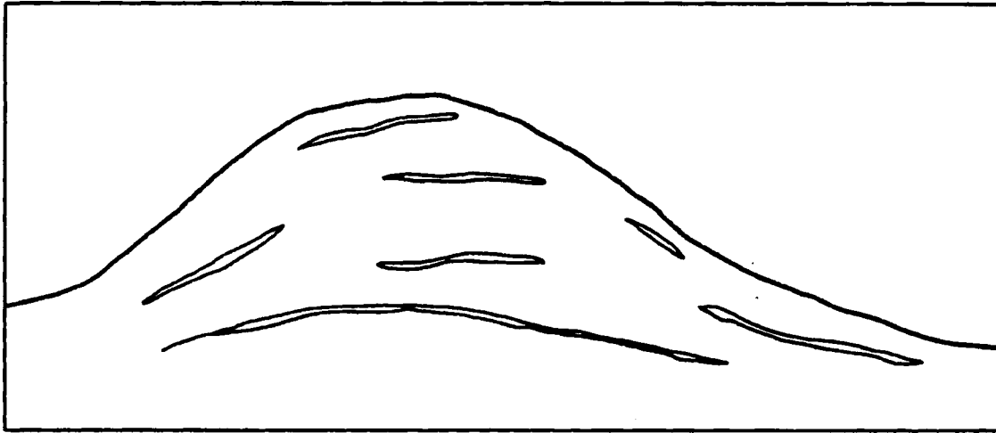
FIGURE 10. Sheet Joints in a Massive Rock Mass (Port-Keller and Gnirk 1981)
