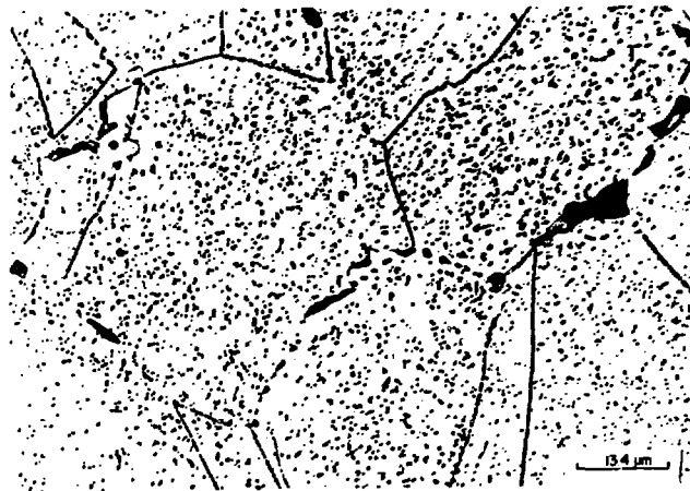
Fig. 10. Optical micrograph showing large amounts of carbide precipitation within the matrix and large sigma phase particles at the grain boundaries in the stressed region of type 304 stainless steel during 73,435 h (8.4 years) at 593°C (1100°F) and 117 MPa.
