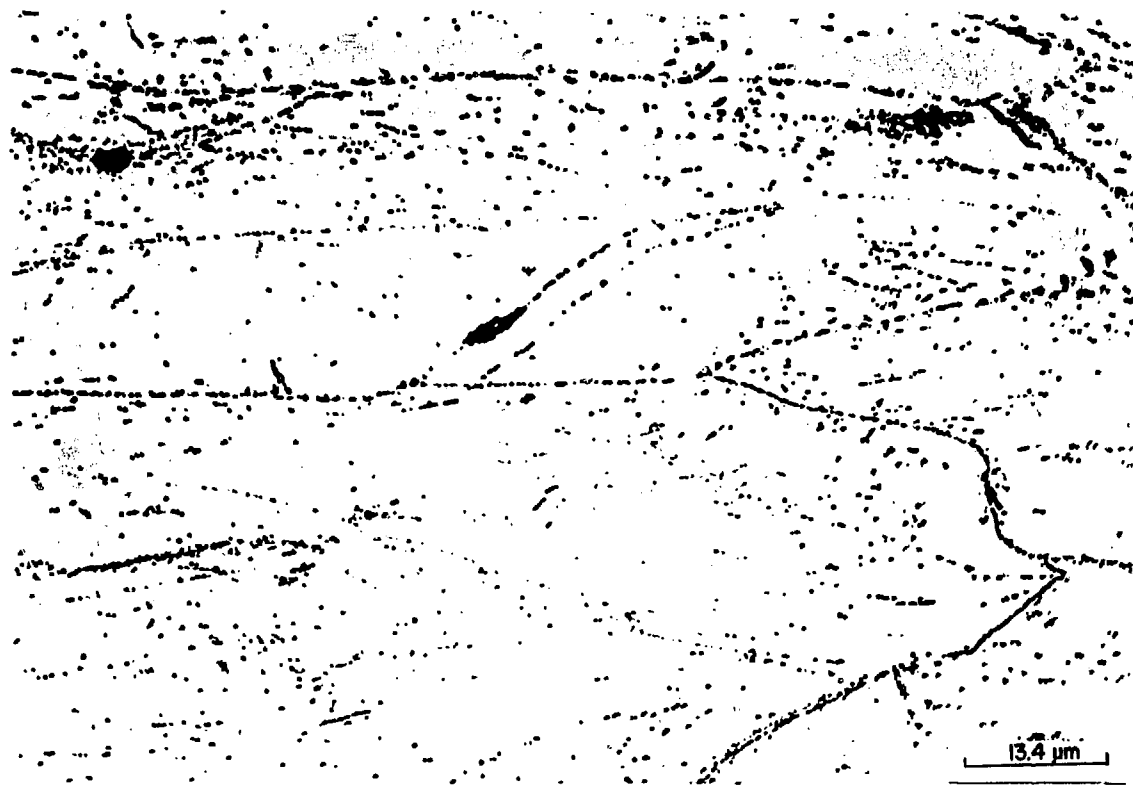
Fig. 16. Optical micrograph of type 316 stainless steel aged for 4.4 \times 10^4 h at 593°C (1100°F) before creep testing. Precipitate structure and mode of failure are the same as for material aged for 10^4 at 593°C (1100°F) shown in Fig. 12.
