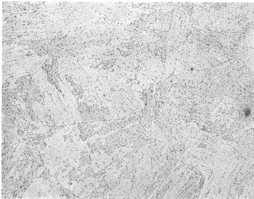
Fig. 4-4 — Microstructure of the center of A542 base plate, Ht. 3707, 500x, Vilella's etchant, CVN = 150 ft-lbs, R_B = 92 .
