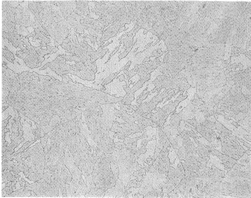
Fig. 4-3 — Microstructure at the center of A542 base plate, Ht. 7868, 500x, Vilella's etchant, CVN = 137.5, R_B = 93
