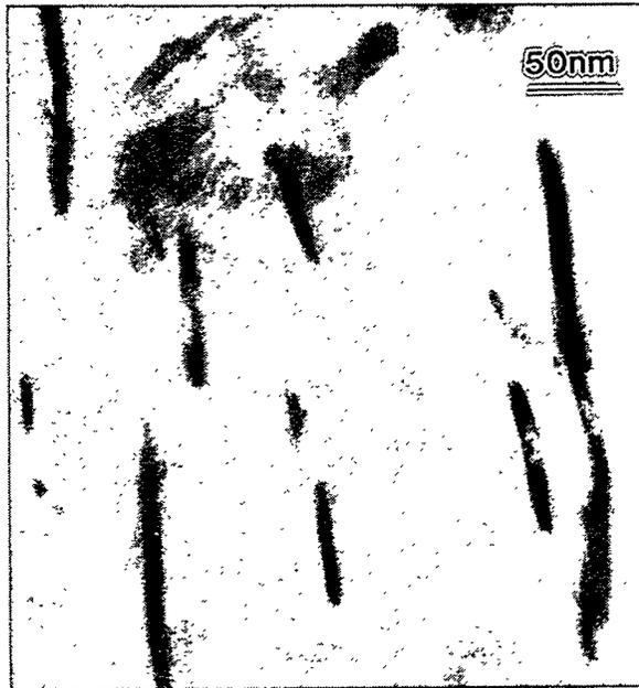
Fig. 4. Micrograph of needle-like carbonitrides in the 7Cr-2WVTa steel.
