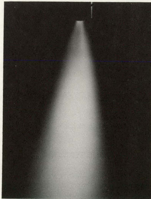
Fig. 3.2. The narrow, well atomized spray pattern provided by the above nozzle permits effective calcination of molten urea solutions.
