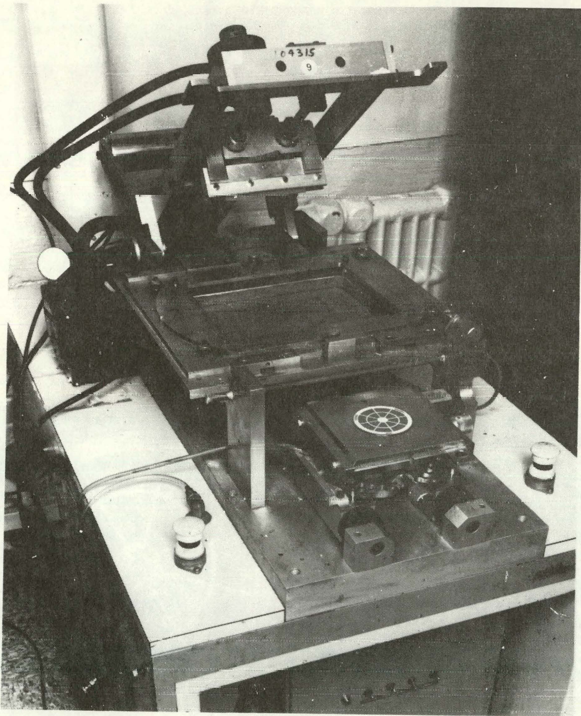
Figure 11. Screening machine and plate details for front of solar cell.
