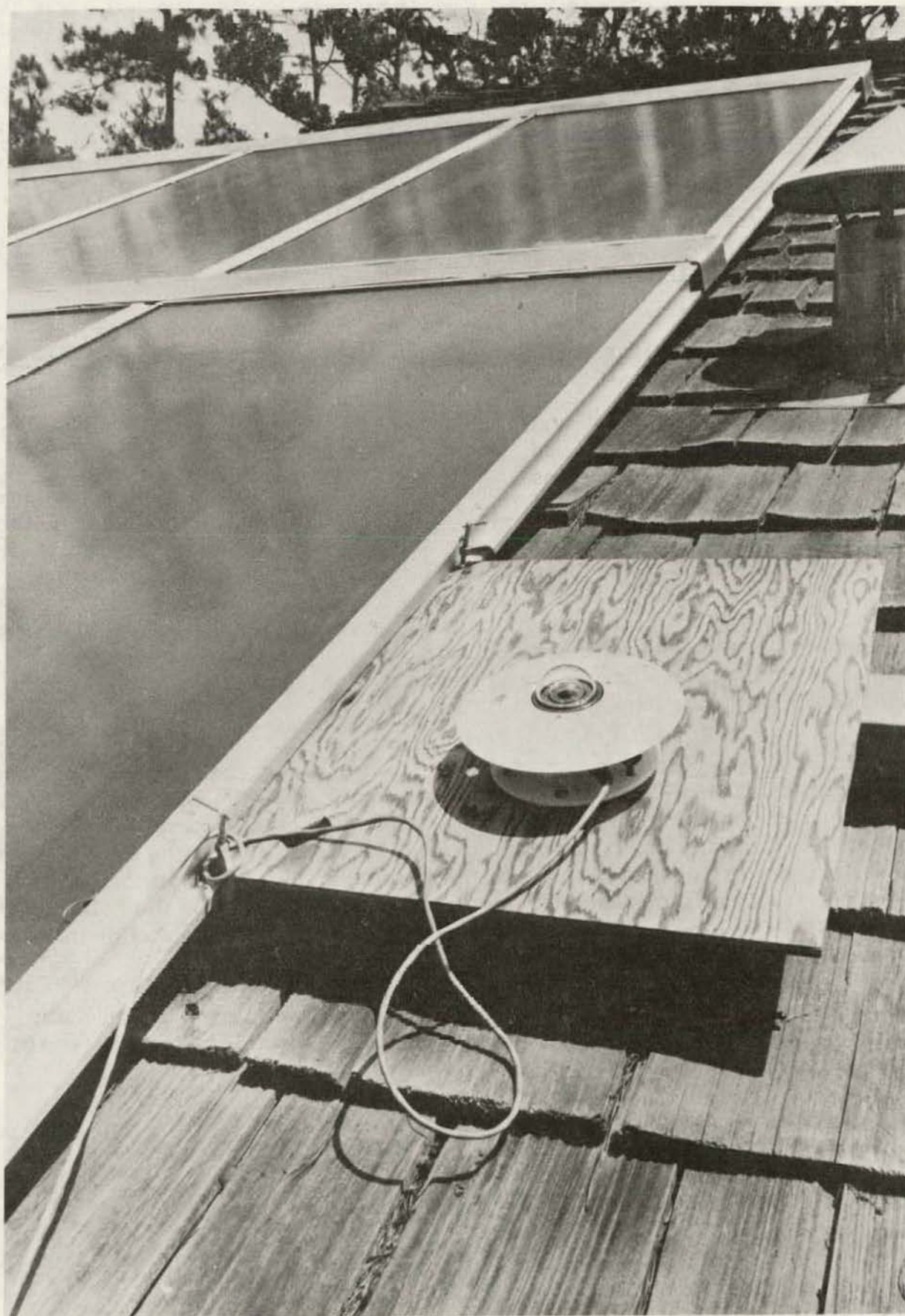
Pyranometer measures sunlight falling on collector, used to determine performance.
