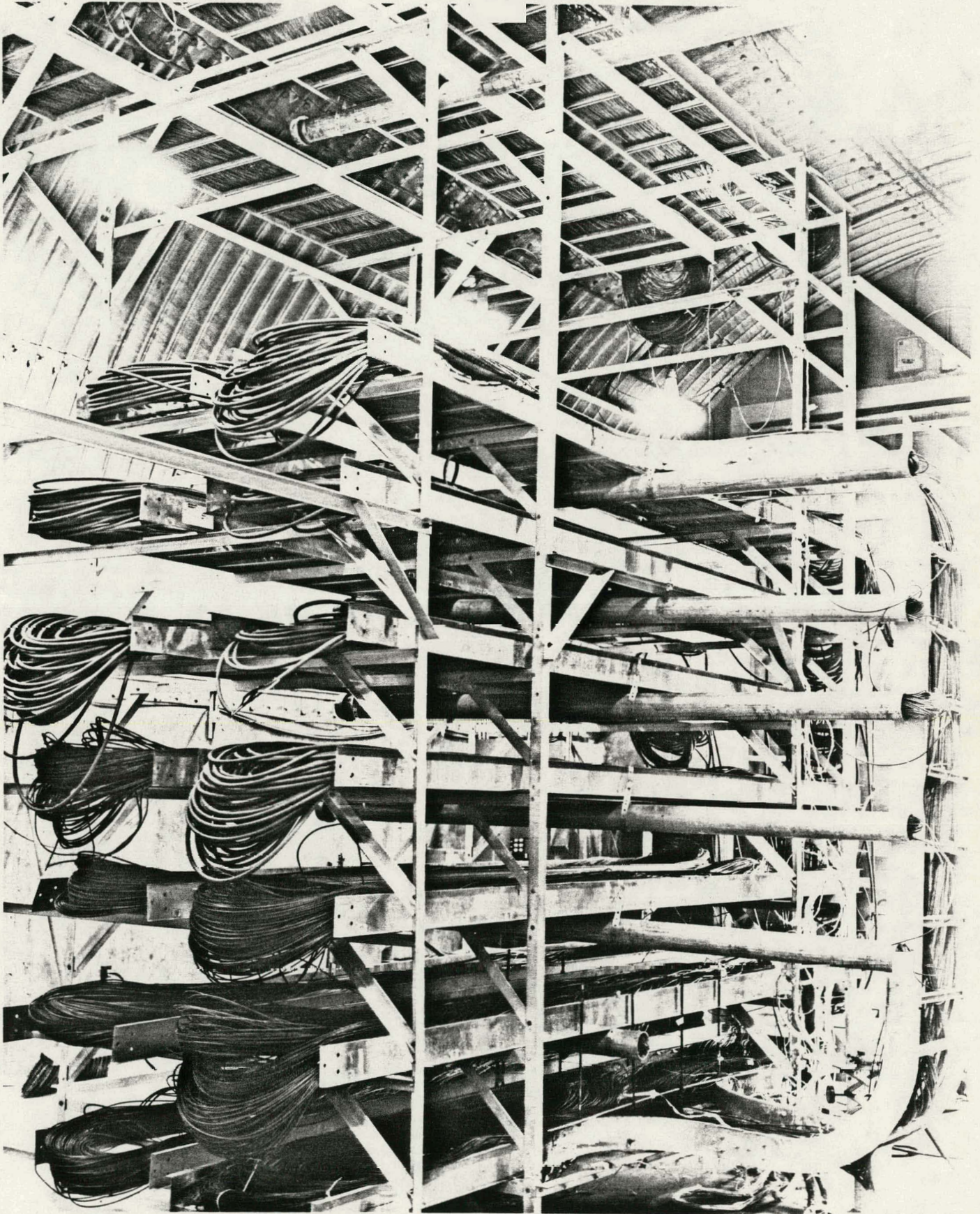
Figure 1. Cable Trays and Conduit loaded with Qualified Cable for Full Scale Exposure Fire Test.
