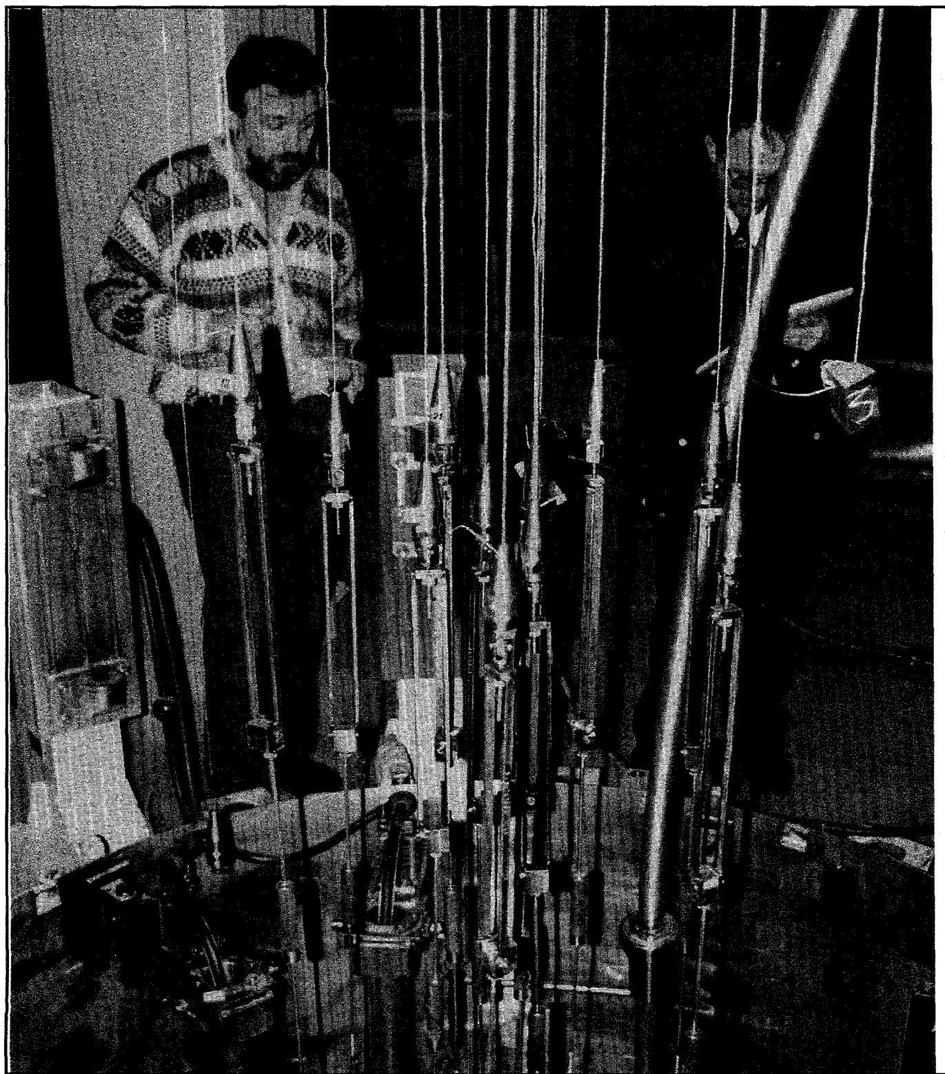
Figure 10.10 View Into the SK-Physical Critical Assembly Core and Control Rod Drive at the Russian Research Center Kurchatov Institute. Criticality studies of extremely tight critical lattices of \text{UO}_2 rods were performed at enrichments greater than 5' and less than about 10-weight percent U-235.
