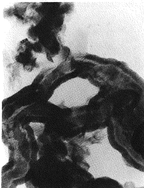
Figure 4-8b. Carbon Formation in Adiabatic Reactor - Carbon Filaments
