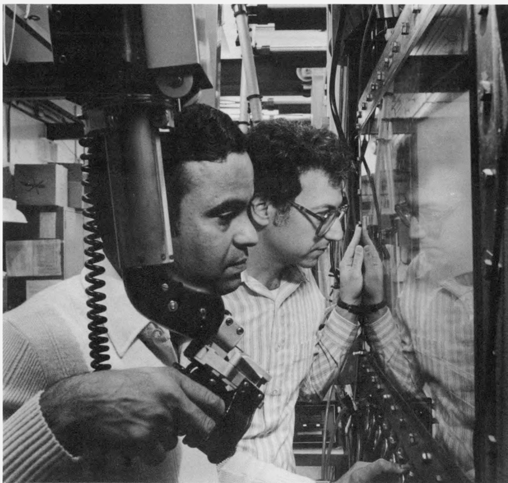
Brookhaven scientists controlling the processing of radioisotopes produced by the Brookhaven Linac Isotope Producer (BLIP). Isotopes for radiodiagnostic and radiotherapy research are produced and developed at Brookhaven. Where commercial facilities for the production of isotopes are not available, they are produced by the BLIP facility for distribution by pharmaceutical companies. Many of these radionuclides have spatial characteristics of properties that make them attractive for use as agents for labeling monoclonal antibodies for both imaging as well as therapy applications.
