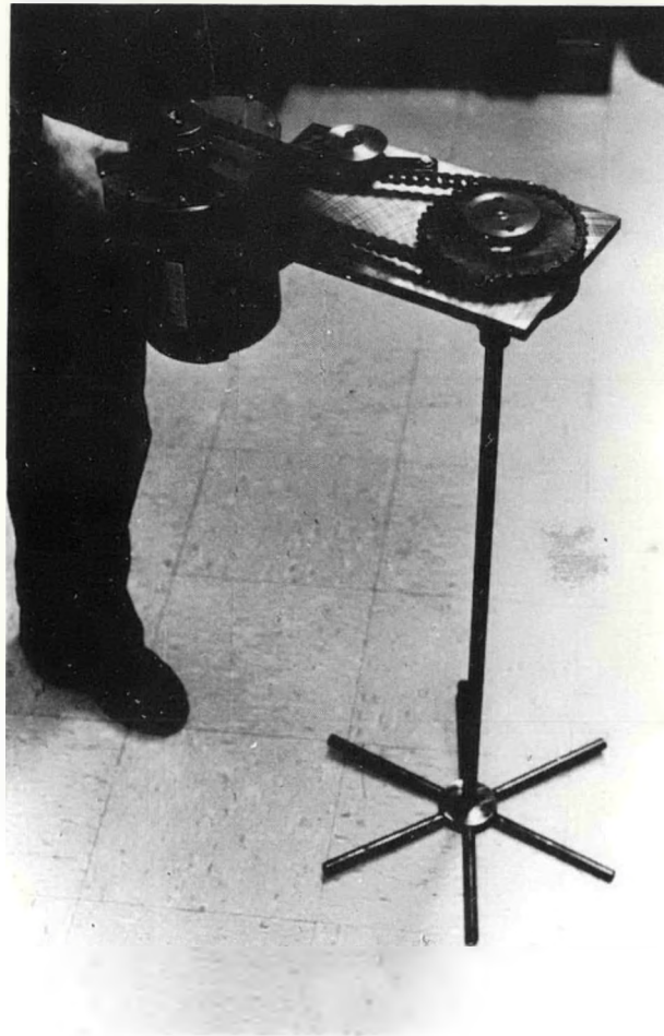
(a) Motor driven stirrer system for coal feeder tank
