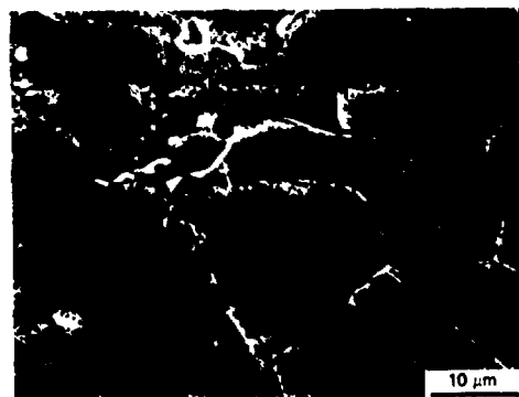
Fig. 7 - Scanning electron micrograph showing massive sigma phase and fine particles of \text{Cr}_{23}\text{C}_6 precipitated in the stressed region of type 304 stainless steel during 6 \times 10^4 h (about 7 years) at 593^\circ\text{C} ( 1100^\circ\text{F} ) and 117 MPa (17 ksi) 12
