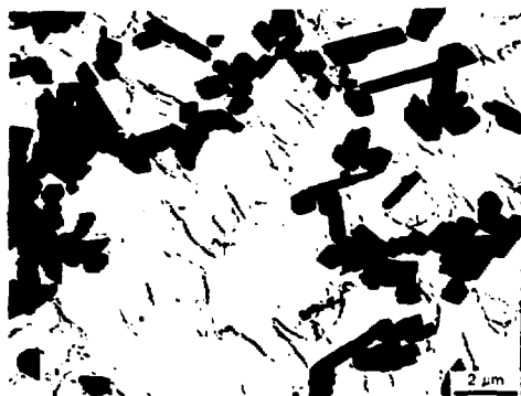
Fig. 6 - Transmission electron micrograph of carbon extraction replica showing forms of \text{Cr}_{23}\text{C}_6 particles extracted from the stressed region of type 304 stainless steel after 6 \times 10^4 h (about 7 years) at 593^\circ\text{C} ( 1100^\circ\text{F} ) and 117 MPa (17 ksi) 12
