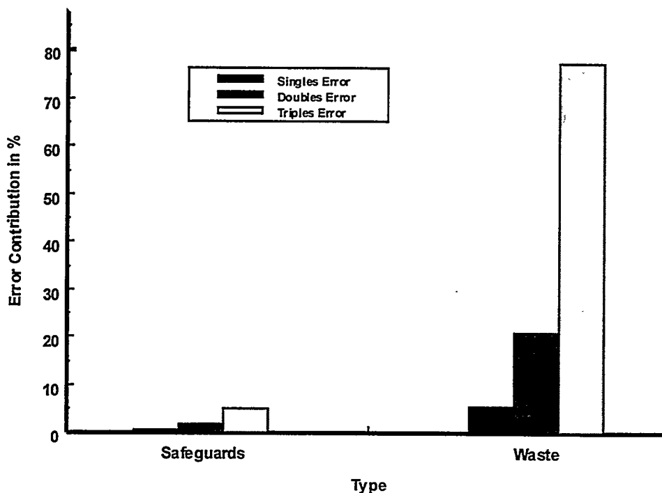
Fig. 4. Multiplicity error sources from singles, doubles, and triples counts for nominal safeguards and waste assay applications, with 20% detection efficiency.
