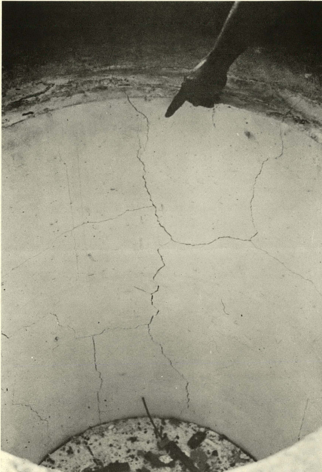
FIGURE 154. As Tested Appearance of Lining #1 After Two Thermal Cycles to 1200° and 2000°F
