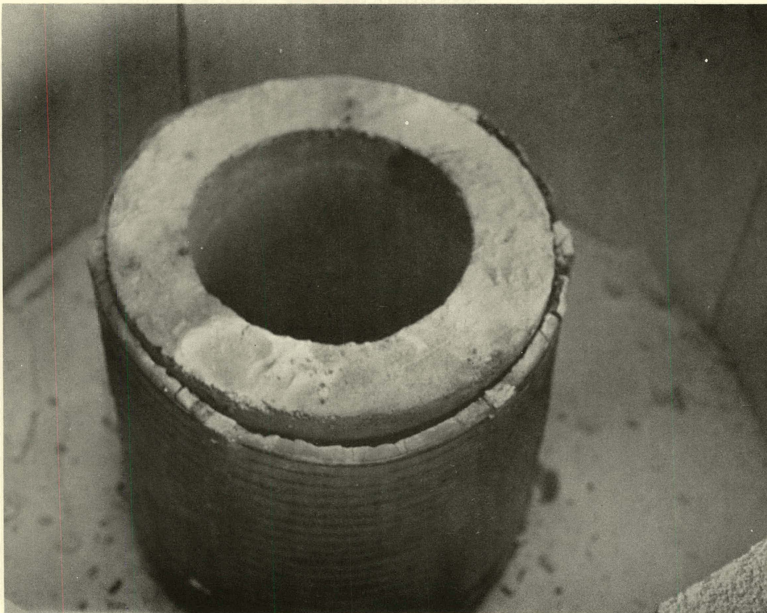
FIGURE 58. Top View of Externally Wound Ceramic Core after Test to 2000°F.
