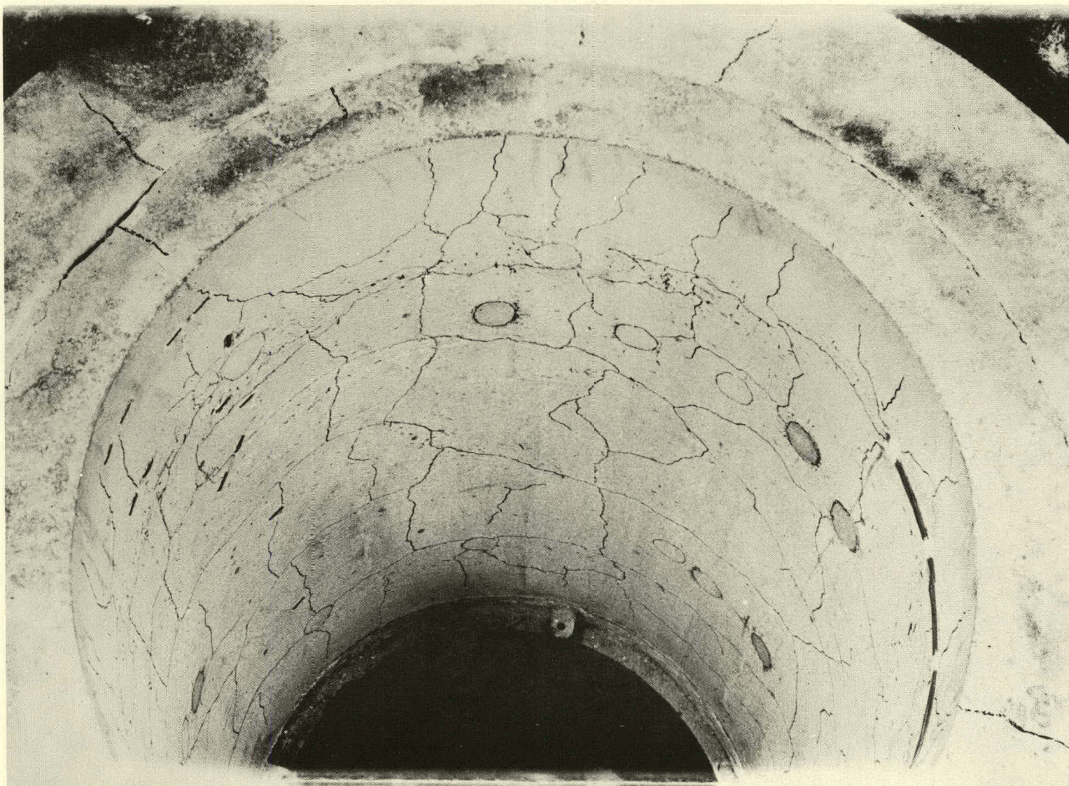
FIGURE 179. Top View of Lining #7 After Three Thermal Cycles (1700°F in Air, 1700°F in 100 psig Air, and 1850°F)
