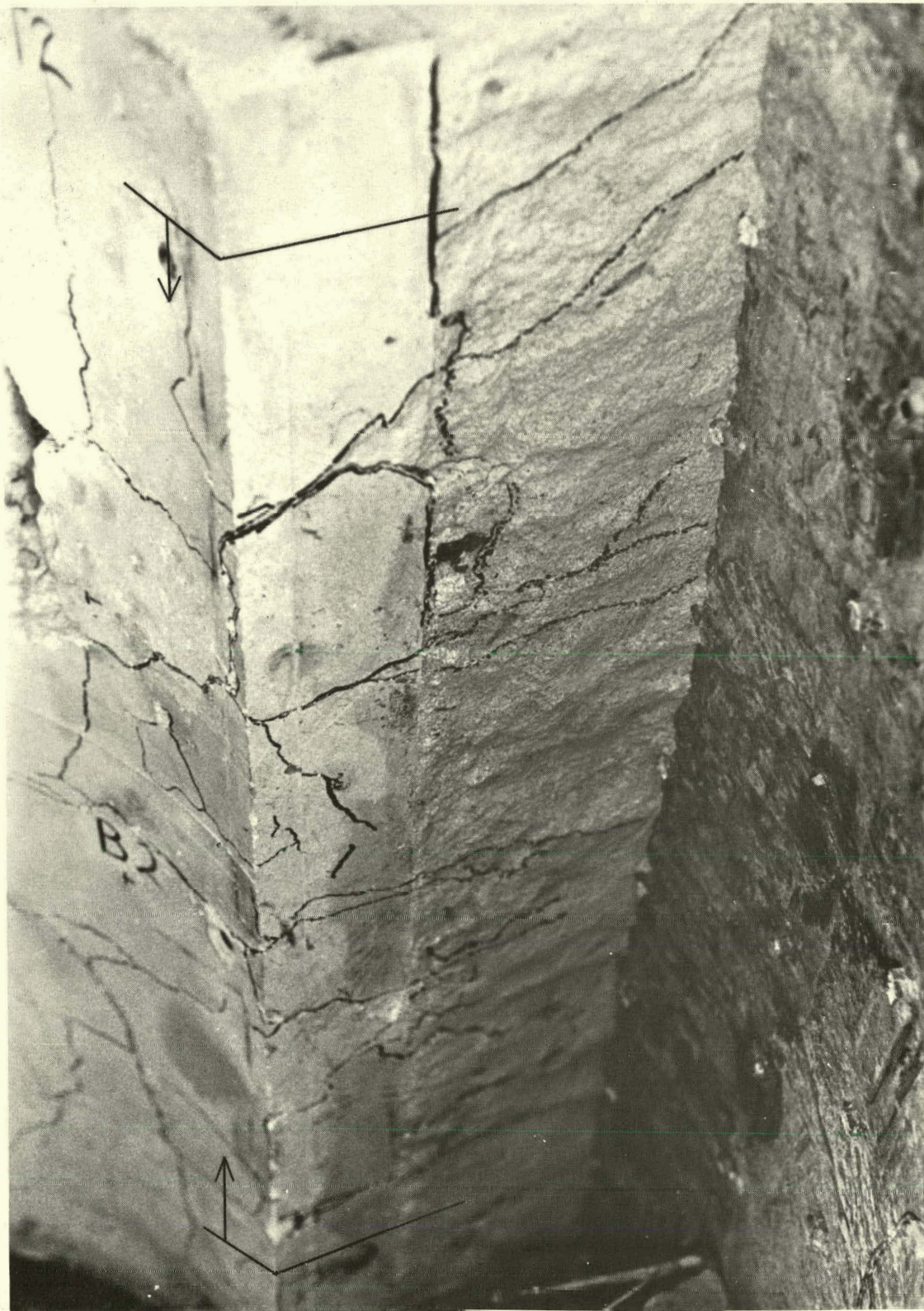
FIGURE 157. Top View of Lining #1 During Tear-Out and Examination. Dense component cut with diamond saw and insulator dressed with a chisel. Cracks are marked with ink. Four foot test zone lies within the arrows.
