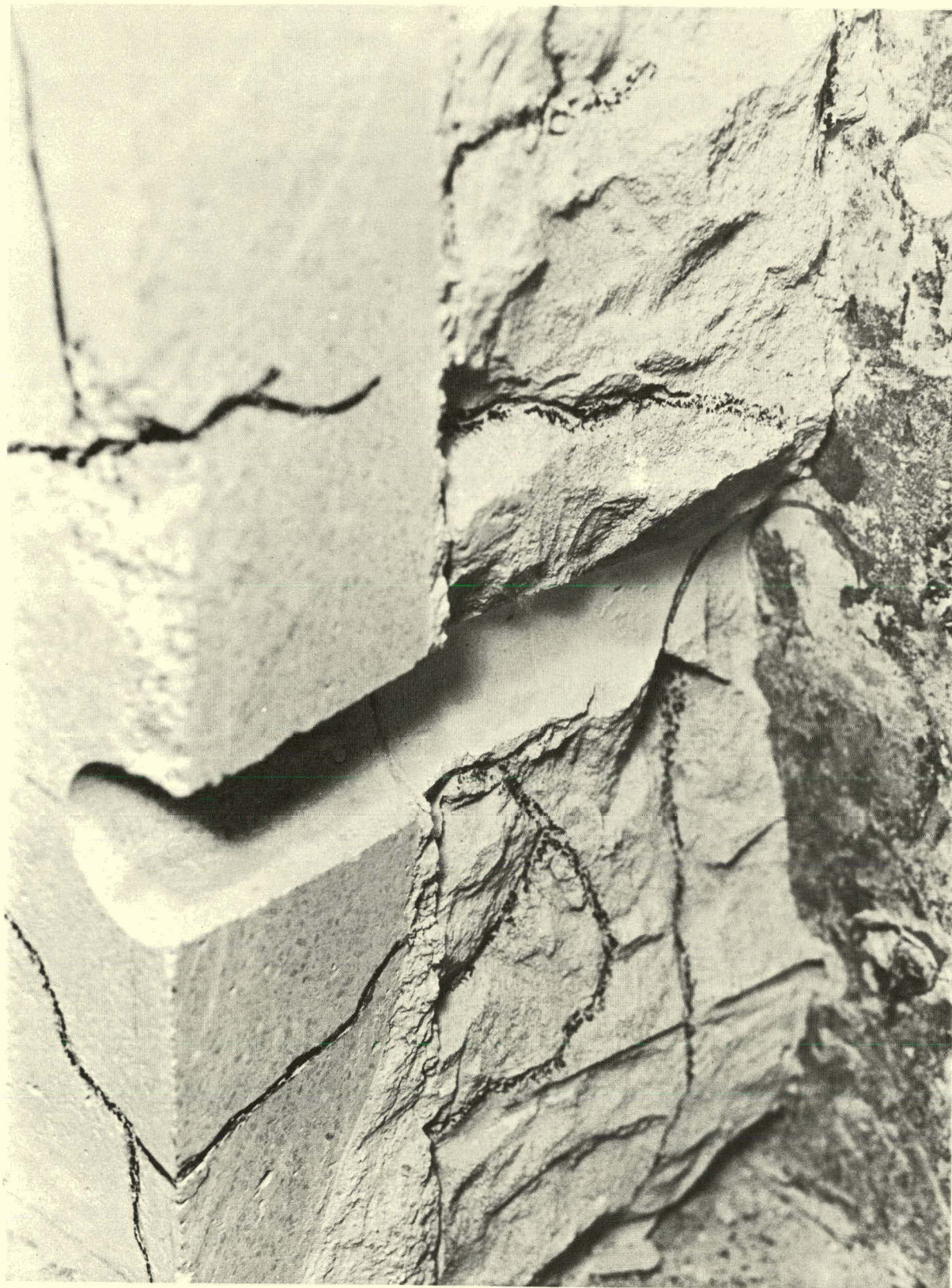
FIGURE 177. Cross Section of Lining #6 After Two Pressurized Steam (120 psig) Heat-Up Tests at 1200 to 1850°F.
