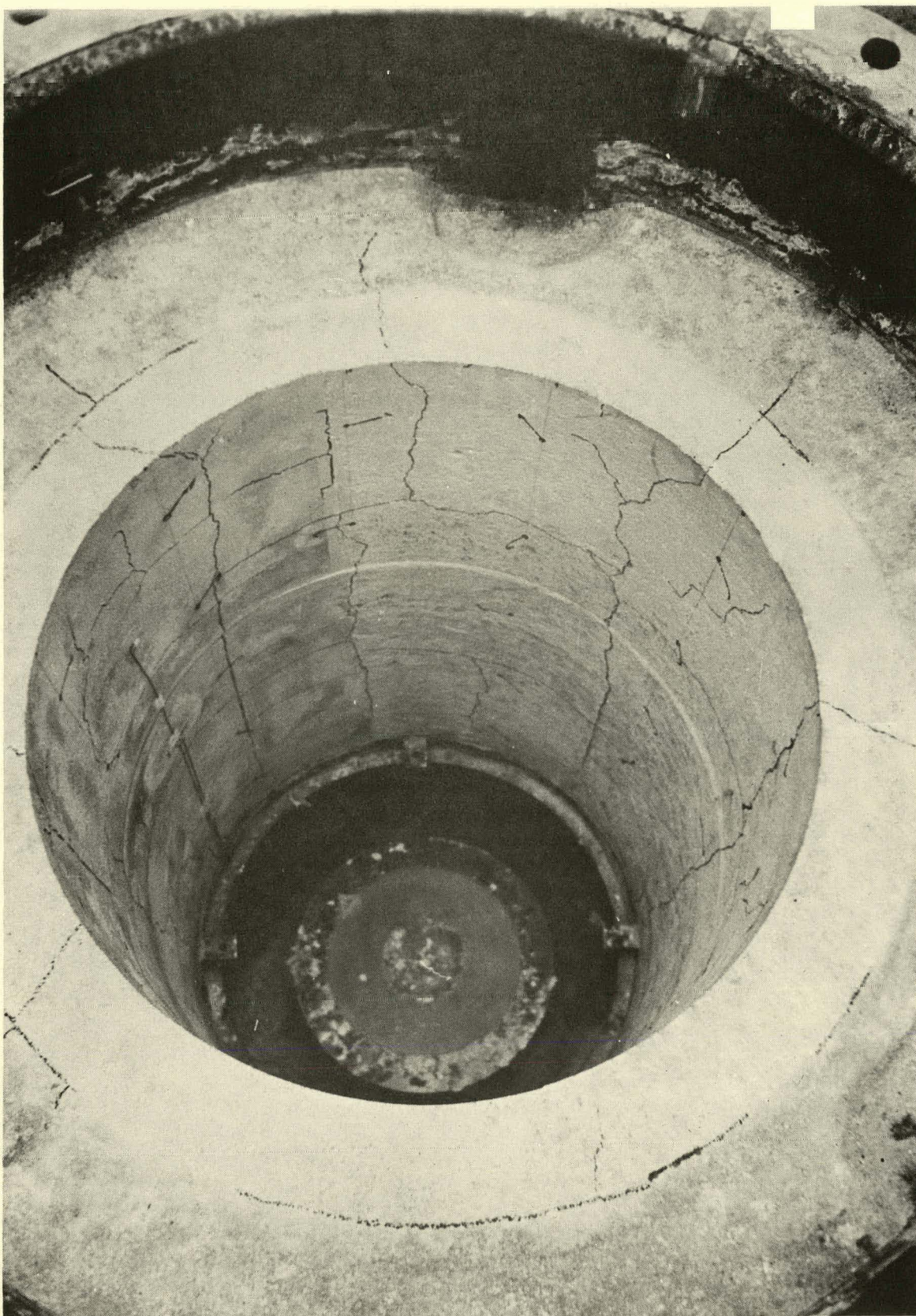
FIGURE 156. Appearance of Lining #2 After Cracks Were Inked Following One Thermal Cycle to 1200°F.
