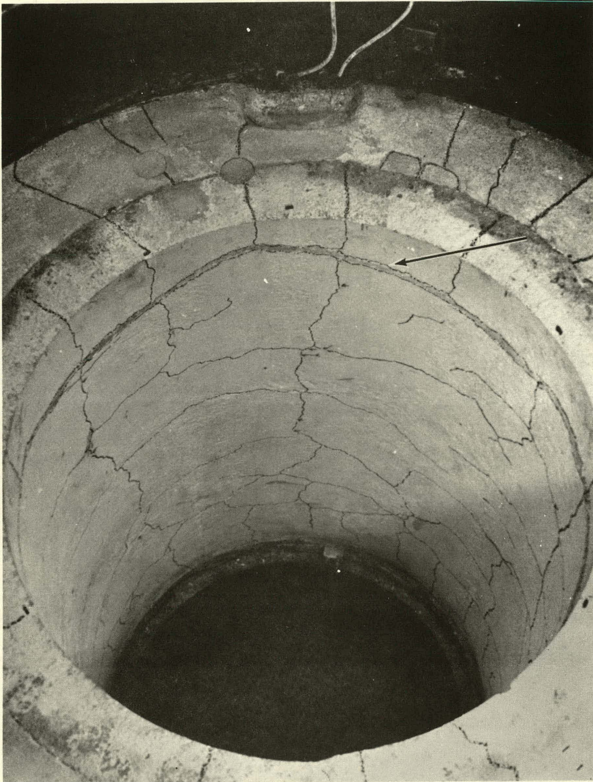
FIGURE 163. Top View of Lining #3 After Heat-up Test to 2000°F
