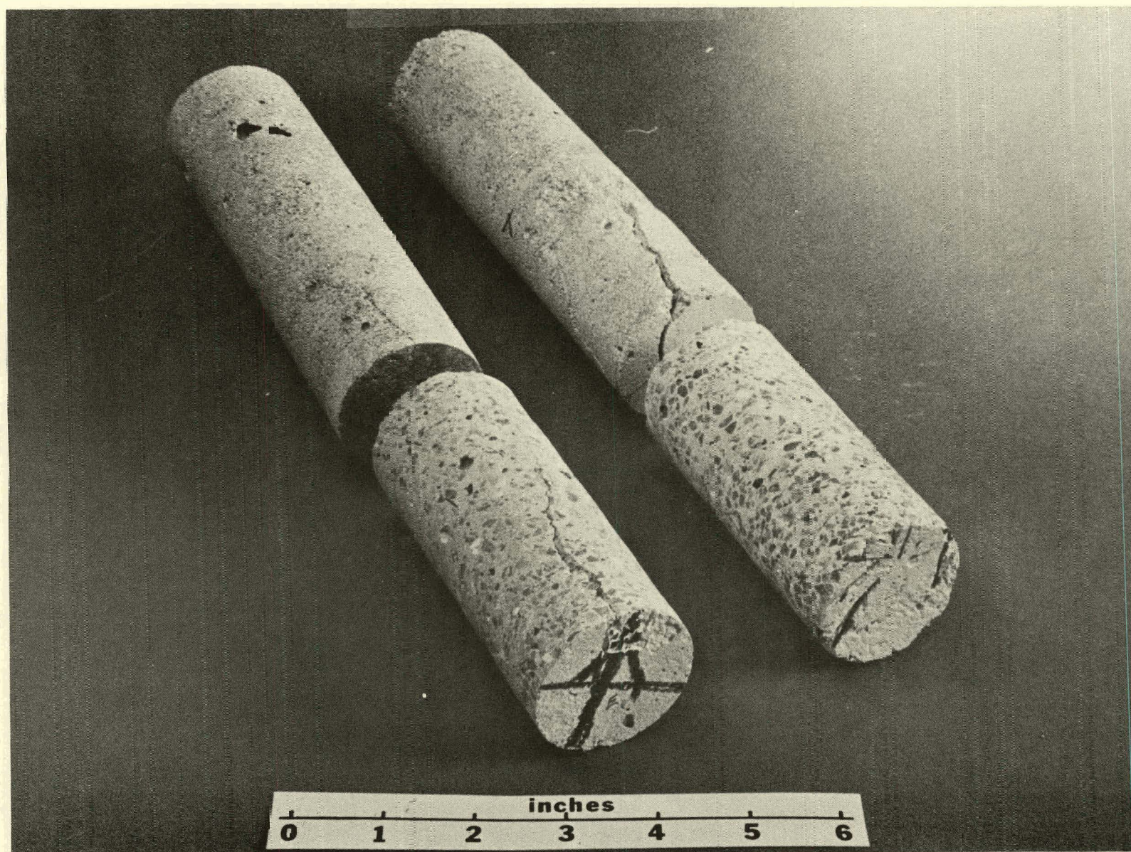
FIGURE 1E9. Drill Cores of Lining #7 and #9 After 1850°F Heat-Up Tests.
