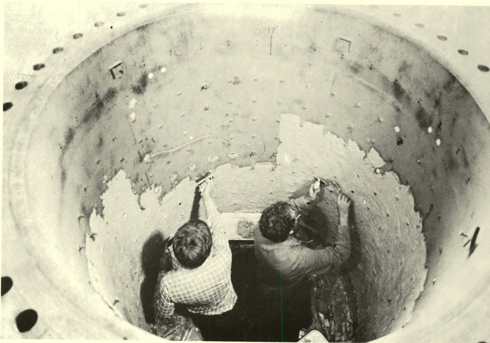
FIGURE 186. Installation Technique Used to Place HES Mortar on Inside of Vessel For Lining #9 Test.
