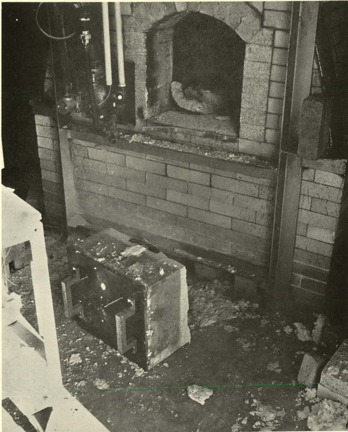
FIGURE 28. Photograph of Panel #5 and Test Furnace After Specimen Failed by Explosive Spalling
