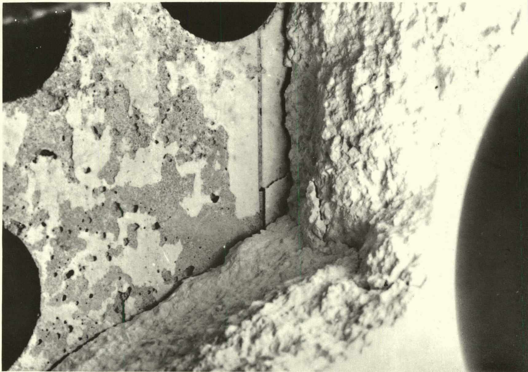
FIGURE 164. View of Dual Component Lining With Section of Dense Component Removed to Show Insulator and Gap at Interface.
