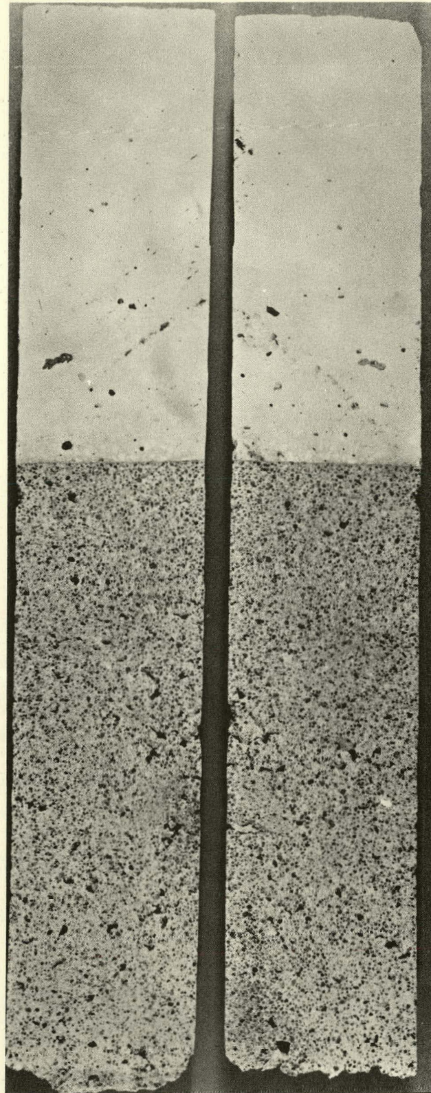
FIGURE 158. Horizontal Cut Through Drill Core Taken From Lining #2 After Test to 1200°F.
