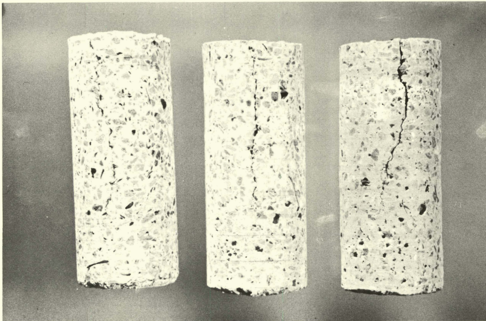
FIGURE 180. Drill Cores of Dense Component Adjacent to Same Vertical Crack (Lining #7 - Three Thermal Cycles).
