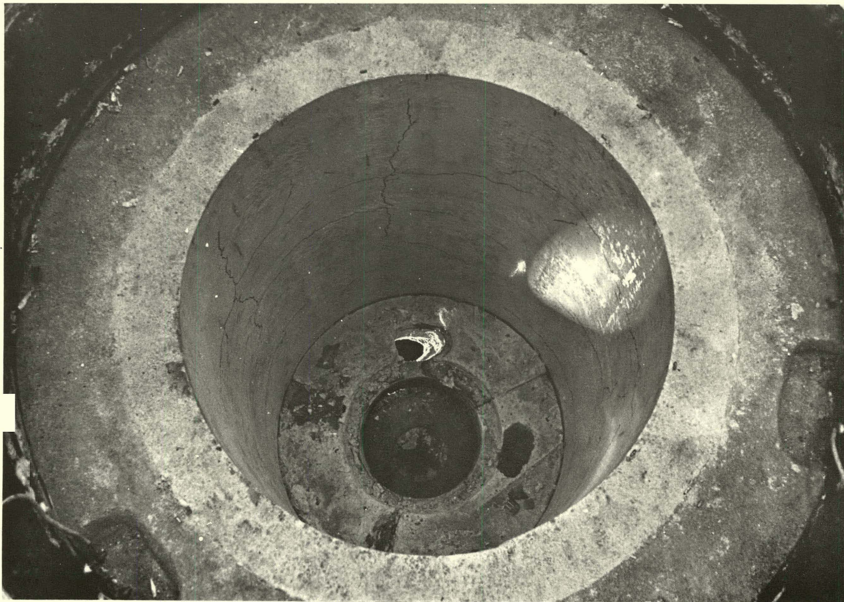
FIGURE 98. Top View of Pressure Vessel/Test Furnace Showing Crack Pattern After Heat-up Test of Lining #3 to 400°F.
