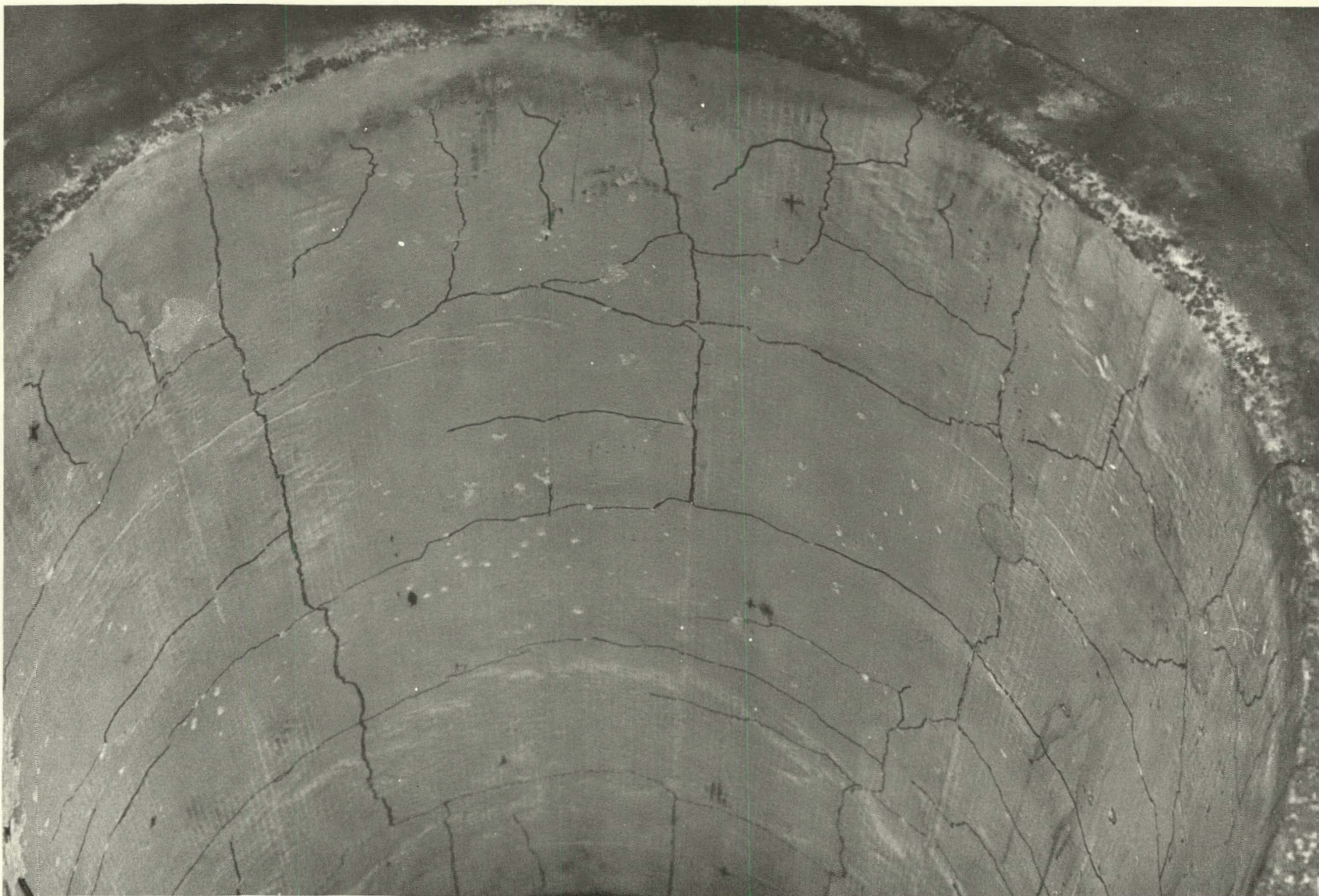
FIGURE 169. Top View of Lining #4 Hot Face After Heat-up Test to 1850°F and 120 psig Steam.
