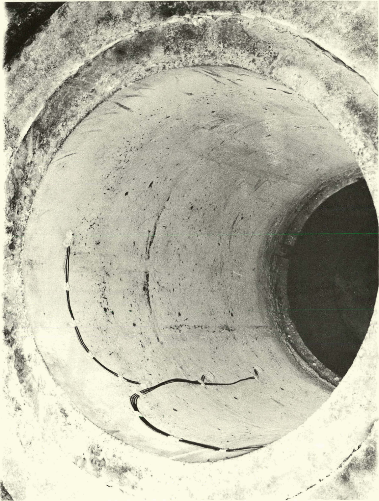
FIGURE 178. Top View of Lining #7 Showing Oxidized Metal Fibers (Dark Spots) After 1850°F Heat-Up Test In Air.
