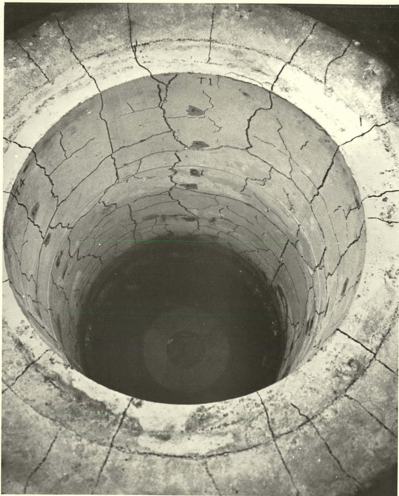
FIGURE 155. Appearance of Lining #1 After Cracks Are Inked Following Two Thermal Cycles to 1200 and 2000°F.
