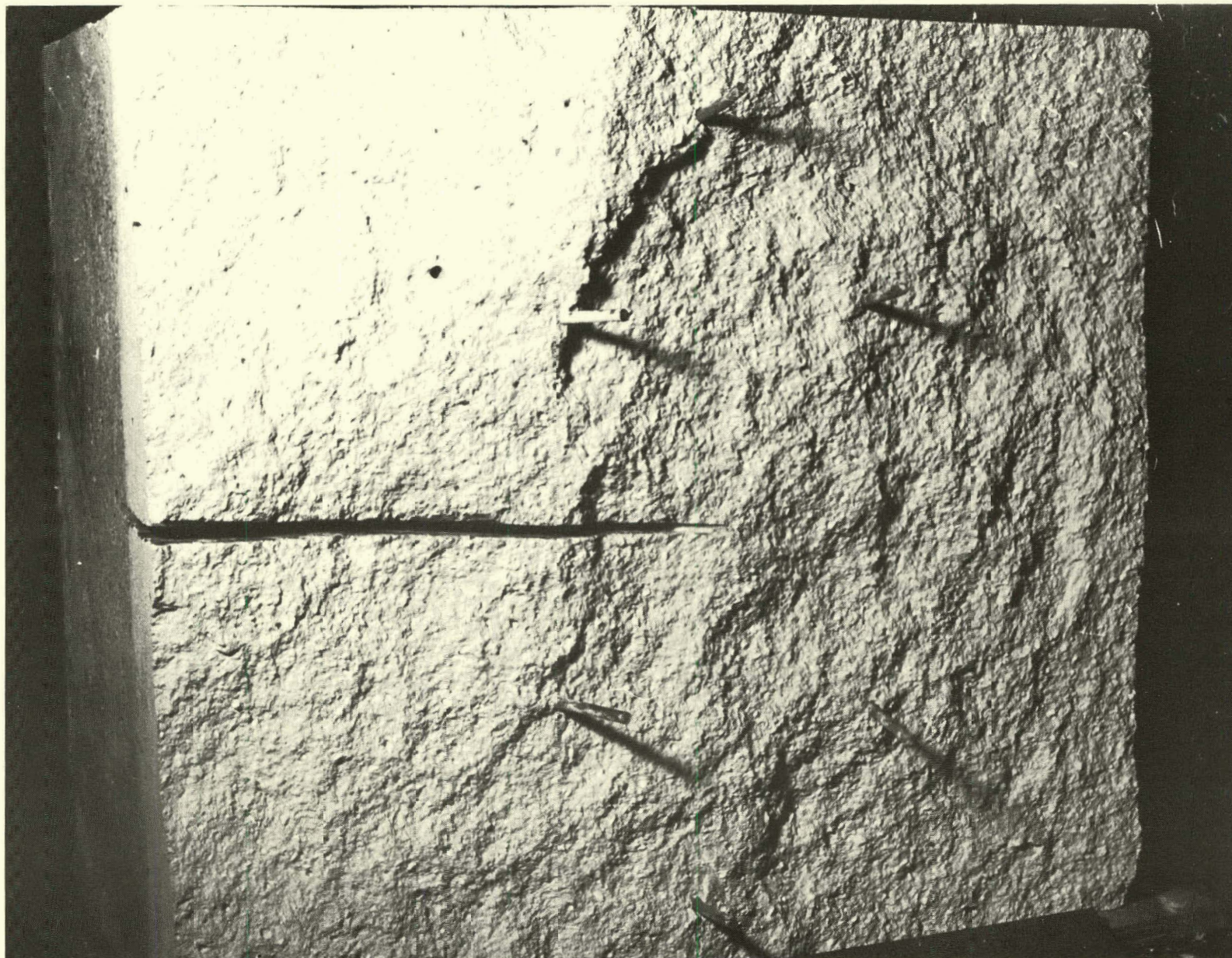
FIGURE 128. Spalled Panel #4. Straight Anchor Sticking Out of Insulator.
