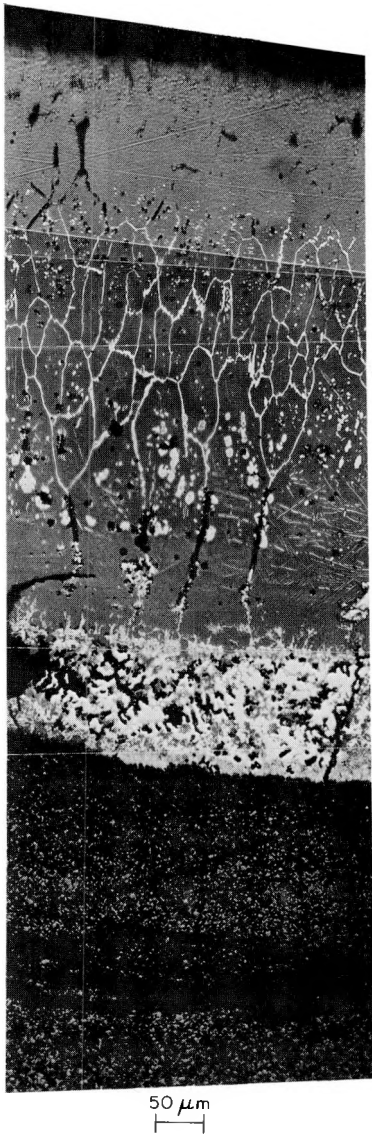
Fig. 15. Structure of Once-liquid Layer between Fuel and Oxidized Cladding. Test HT-2. Neg. No. 222573.
