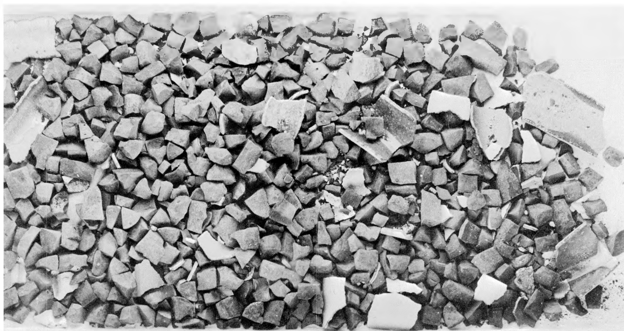
Fig. 9. Small Fuel and Cladding Pieces of the HT-2 Test Specimen. Neg. Nos. MSD-222018 and -222019.
