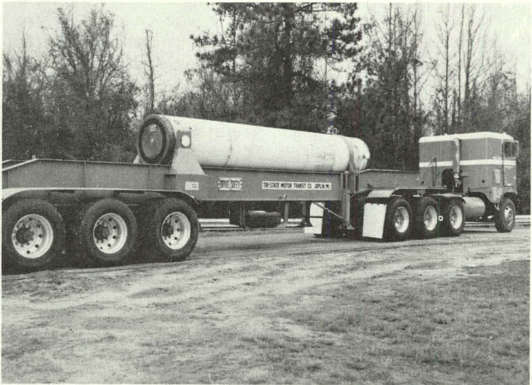
FIGURE 18. Truck Cask Loaded on a Special Trailer
