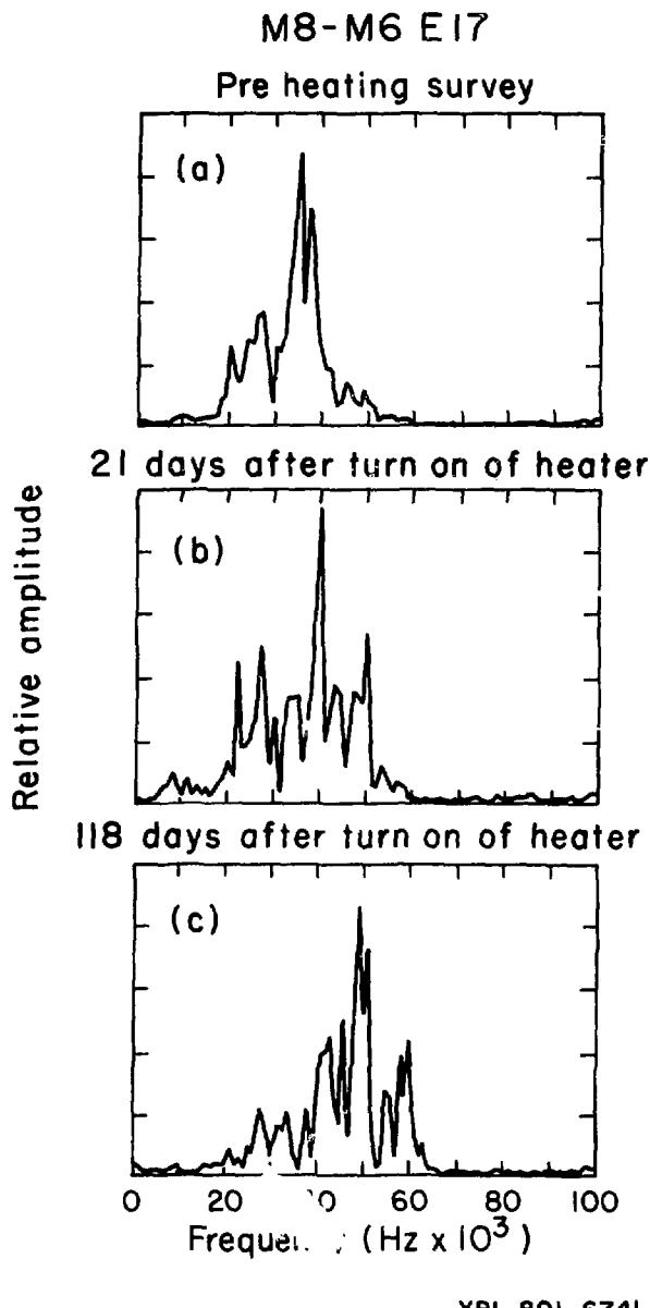
Fig. 9. Amplitude spectra of between-hole survey before and after heater turn-on.
