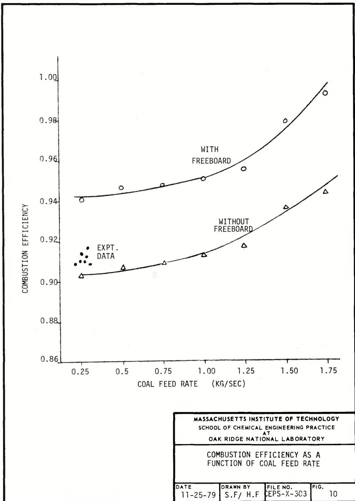
2. The freeboard model slightly increases the prediction of combustion efficiency.
