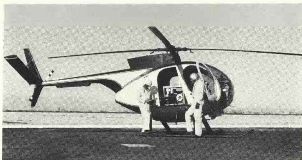
Figure 5. HUGHES H-500 SURVEY HELICOPTER The Hughes H-500 is an excellent aerial platform for small survey sites. Twenty NaI detectors are carried in two pods on the sides of the aircraft. The REDAR system is mounted in the rear half of the passenger compartment.
