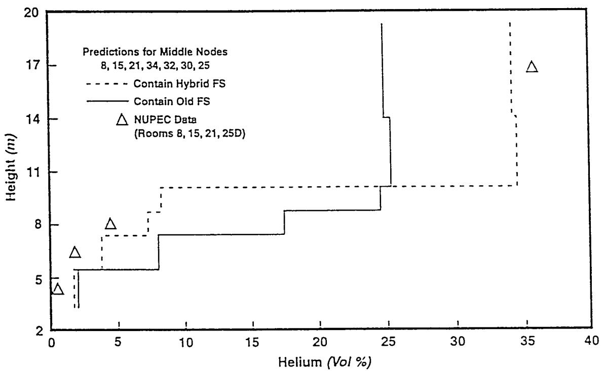
Figure 1. The Helium Concentration Profiles Predicted in the NUPEC M-8-1 Experiment at the End of the Injection Period, Compared to the Experimental Data.
