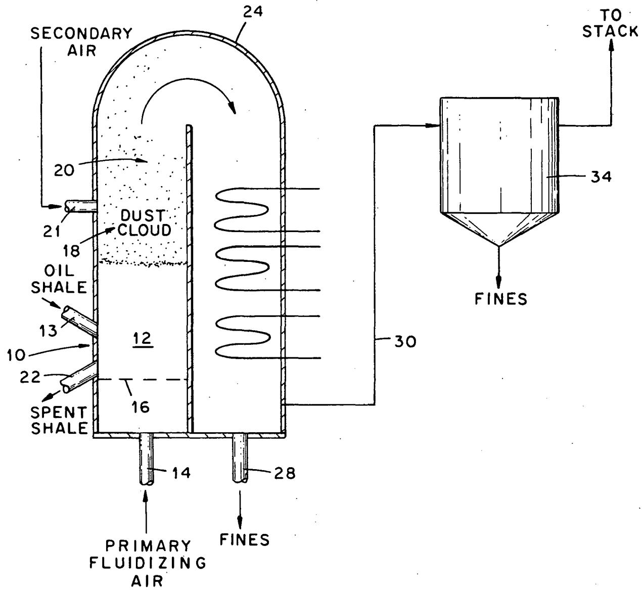
radiated back down into the retorting zone 12 of the fluidized bed so as to facilitate the extraction of the volatile hydrocarbons from the oil shale. The spent shale is removed from the fluidized bed 10 by a suitable conduit as shown at 22.
