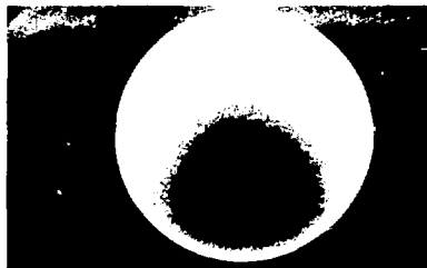
Figure 34. SEM photograph of a PVA microsphere coated via plasma polymerization with \sim 16 \mu\text{m} of CH coating. The coating work was carried out by Letts and Corley at LLNL. 40
