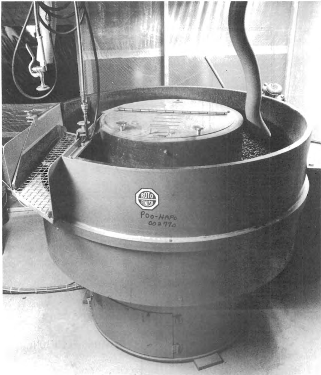
FIGURE 3. Annular Vibratory Finisher with 12-ft 3 Capacity
