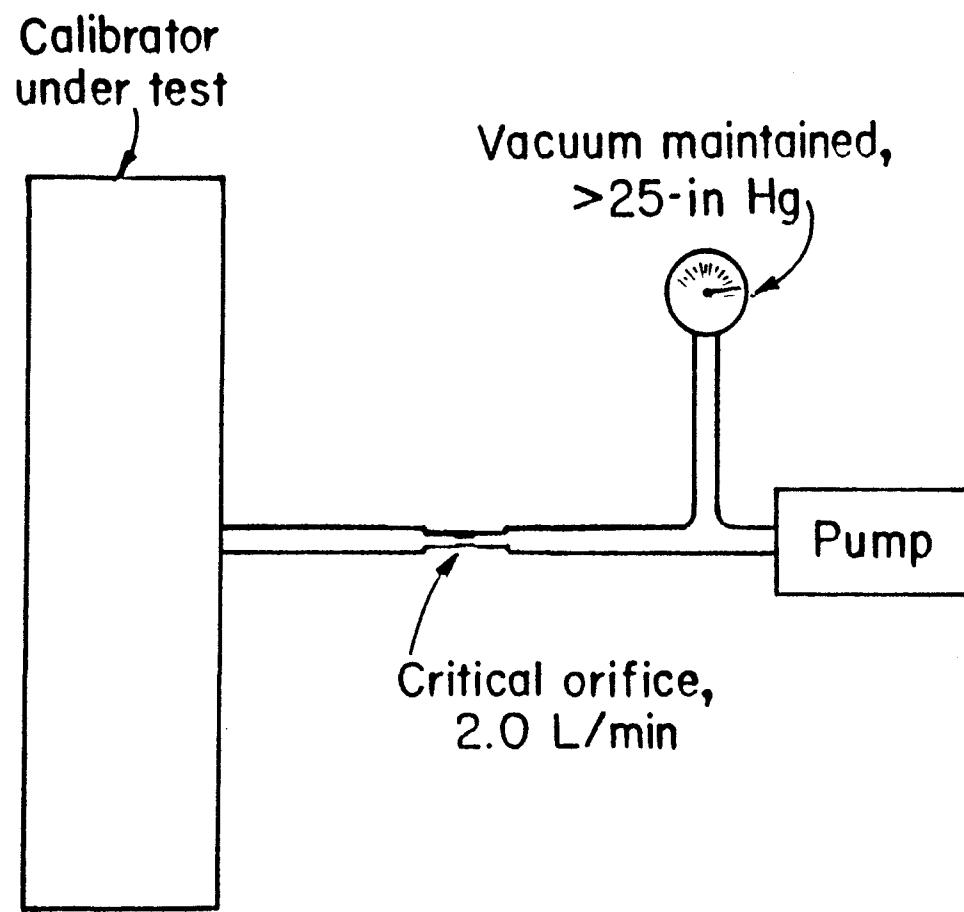
Figure 1. - Schematic - Experimental Setup
