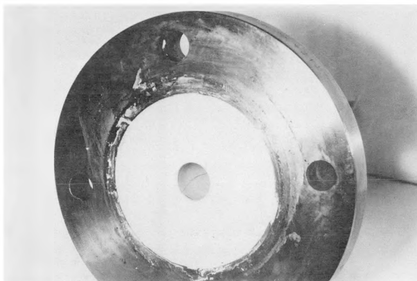
TITANIUM REBOILER TUBE SHEET EXPOSED TO LWR WASTE SOLUTION
