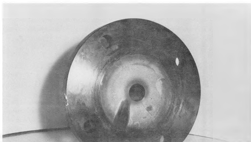
TITANIUM REBOILER TUBE EXPOSED TO 7-MOLAR NITRIC ACID
