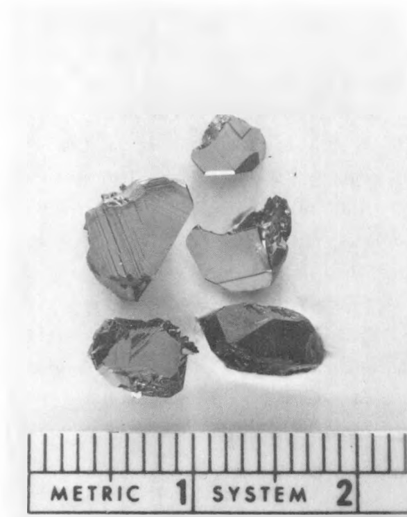
Figure 2.18 Several Large Single Crystals of RuO 2 Grown at Brooklyn College by the Chemical Vapor Transport Method
