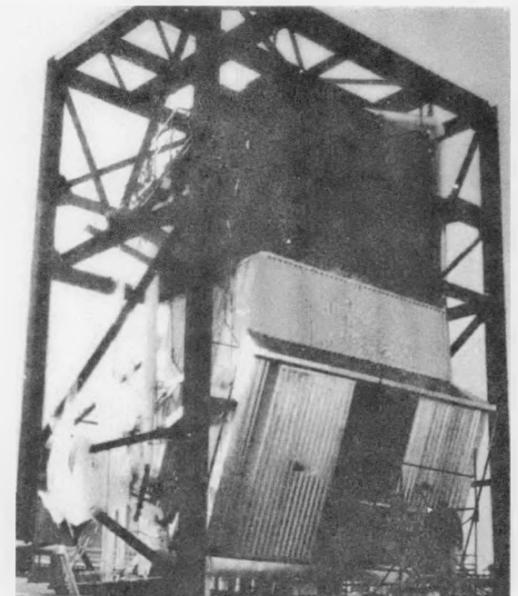
(c) 5 MW e Receiver Built for Subsystem Research Experiment
