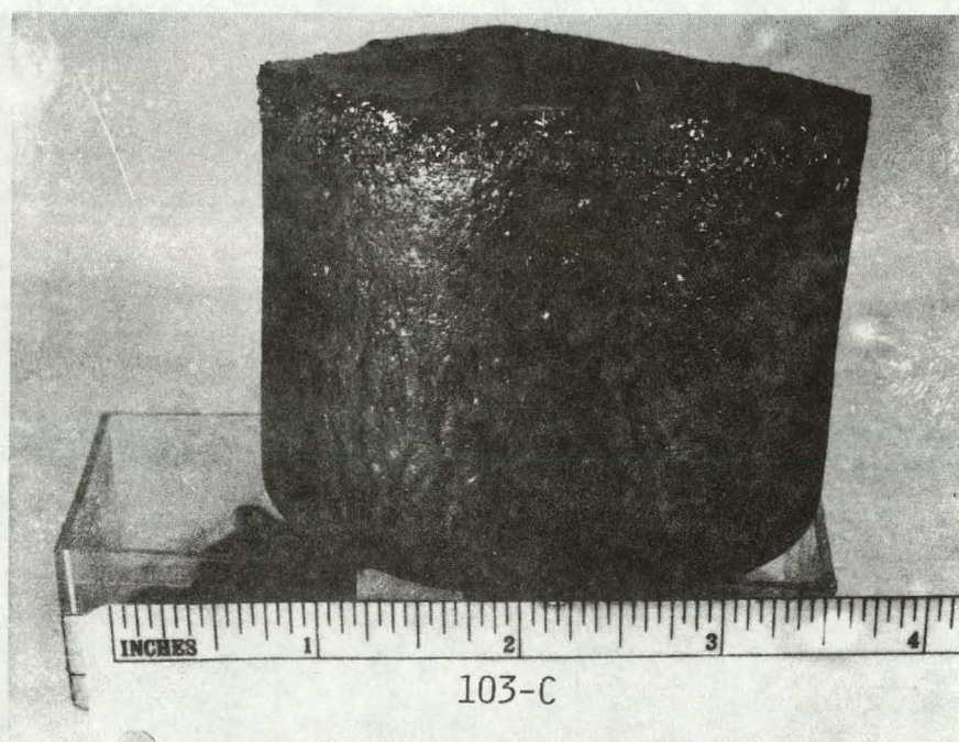
Figure 15. Polished and Etched Section of Boule 109-C Showing Melt-back and Growth on the Sides of the Seed. The effect of insulation can be seen in the top section.
