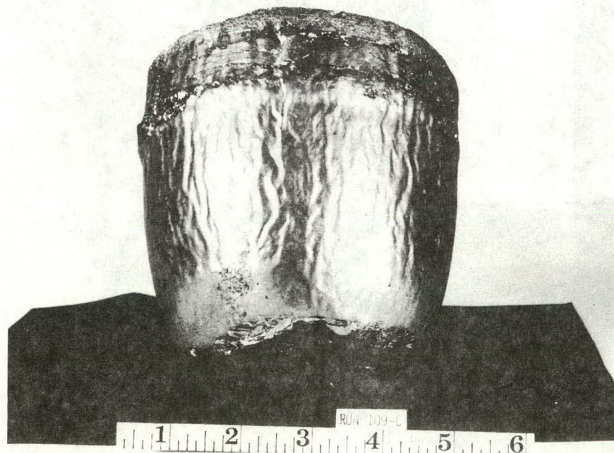
Figure 14. A crack-free 3.3 Kg silicon boule cast in run 109-C
