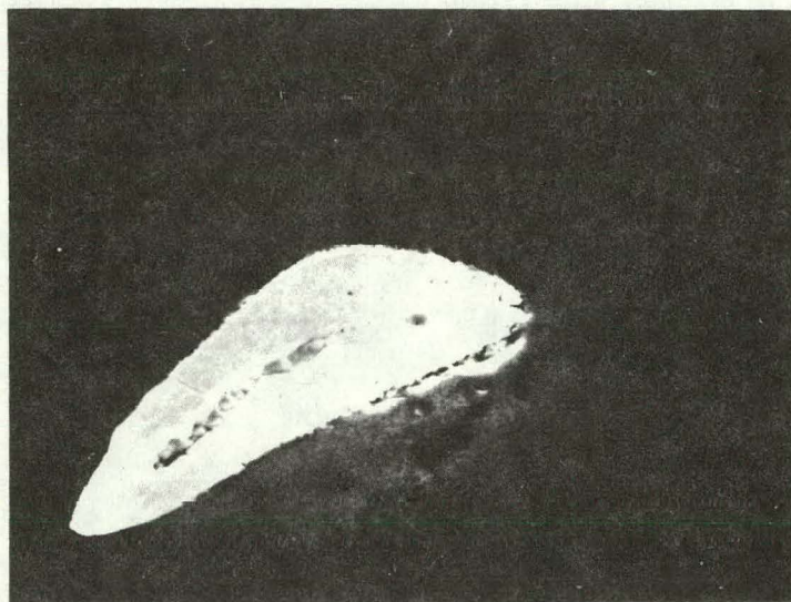
Figure 3 Blade-like Mn_{11}Si_{19} second-phase particle identified by EDAX analysis of ingot W226Mn-010.
