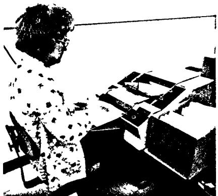
Cartridge of microfilm film is blip coded for retrieval.
