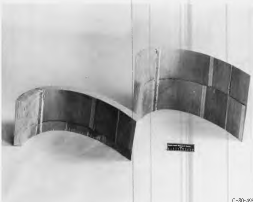
Figure 41. - Internal surface view at point of leading-edge penetration. (From ref. 4.)
