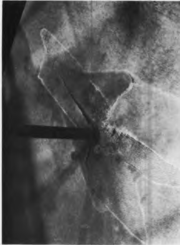
Figure 44. - Aftermath of high-current passage through Nomex after-body panel. (From ref. 4.)
