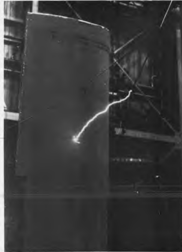
Figure 35. - Penetration at afterbody panels. (From ref. 4.)
