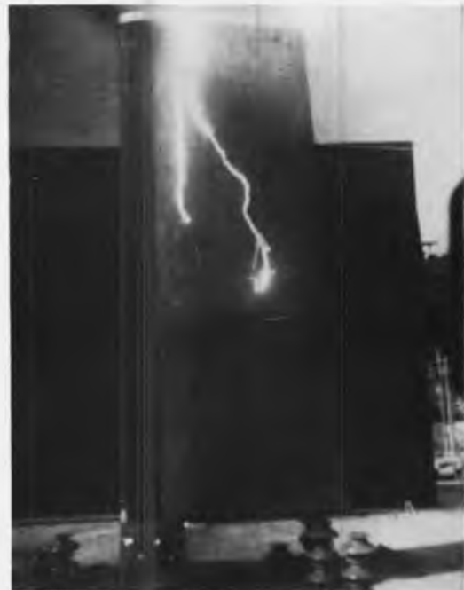
(b) Attachment on cap surface with external flashovers to metal base.
