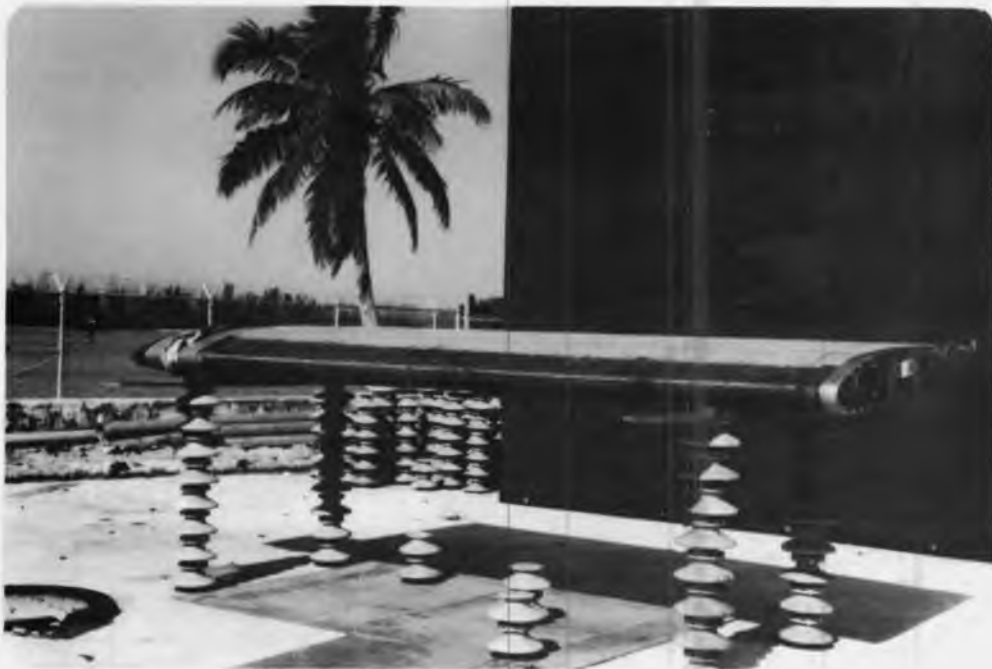
Figure 20. - Lightning accommodation system concept for Kaman blade design.
