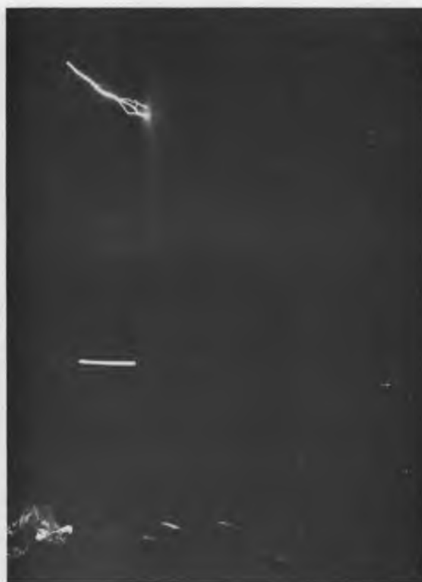
Figure 29. - Attempted attachment to leading edge (actually attaching to screen). (From ref. 4.)
