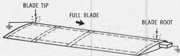
Figure 17. - Kaman test specimen arrangement for high-current damage tests. (From ref. 3.)
