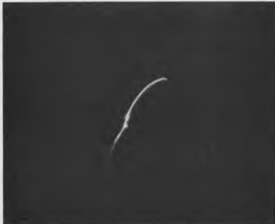
(c) Interior streamering in leading-edge span.
