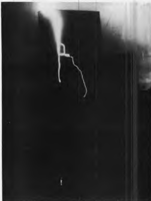
(e) Attachment at tip with external surface flashover and internal stitching (streamering).
