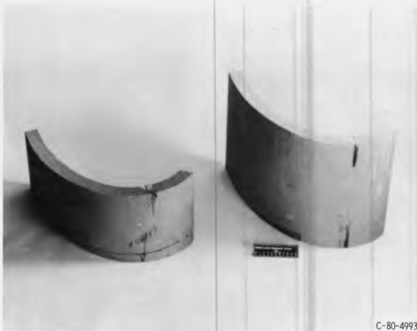
Figure 40. - External surface view at point of leading-edge penetration. (From ref. 4.)
