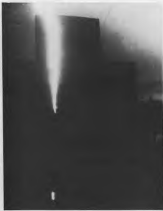
(d) Attachment at tip with external surface flashover followed by stitching and resurfacing.
