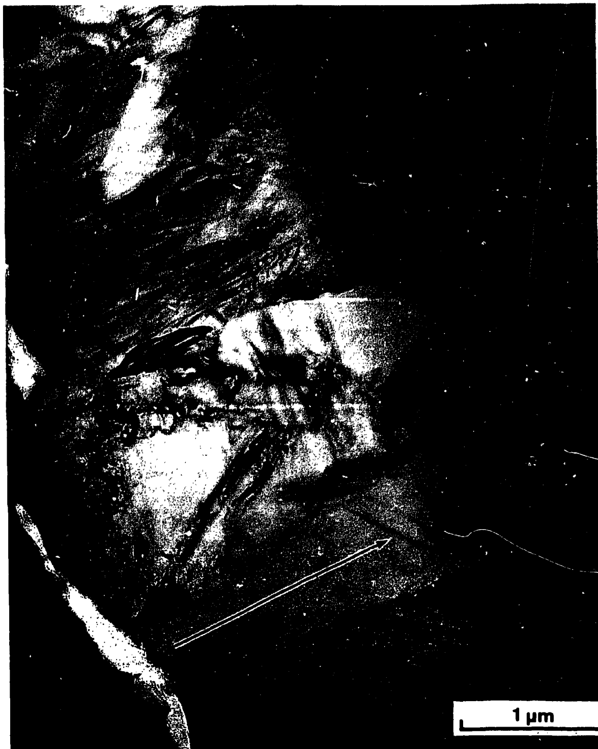
Fig. 8. Microstructure of SiC coating Ag-1, on \text{UO}_2 + \text{Ag} kernel, after 2000 h at \sim 1475^\circ\text{C} . No second phases or grain boundary films could be seen. Arrow indicates radial outward direction of SiC coating.
