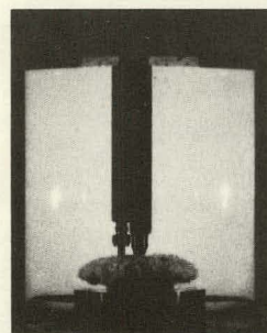
t = 3.375 ms \Delta t = 2.060 ms Bubble reaches pressure transducer
