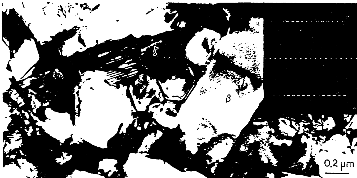
Figure 5. TEM image of sample #H showing elongated \beta' grains as well as elongated and highly faulted \zeta - \text{Si}_3\text{Al}_7\text{O}_3\text{N}_9 grains (labelled). Diffraction pattern of a \zeta - \text{Si}_3\text{Al}_7\text{O}_3\text{N}_9 grain is inset.
