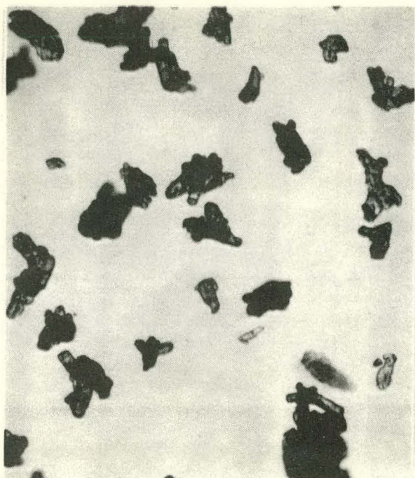
Sample Size 1.1 grams TATB Retained by 44 µm Sieve
