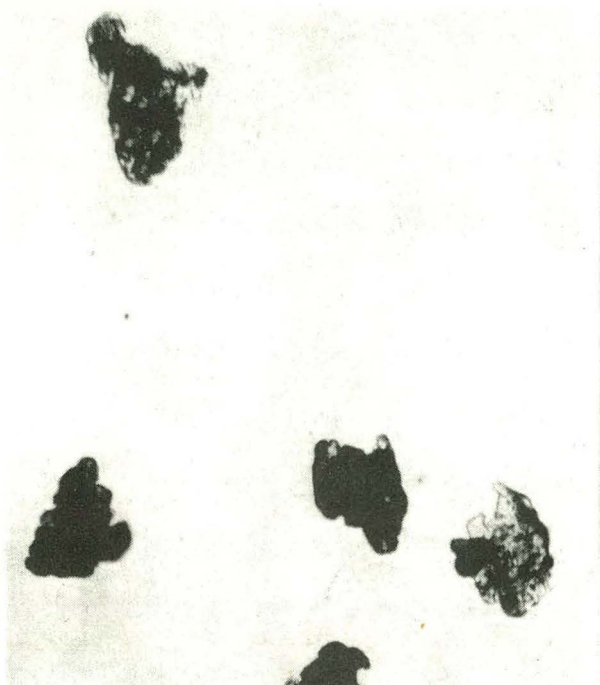
TATB Retained on 80 \mu m Sieve Before 100 Watt Ultrasonic Treatment (Mag. \sim 135X)
