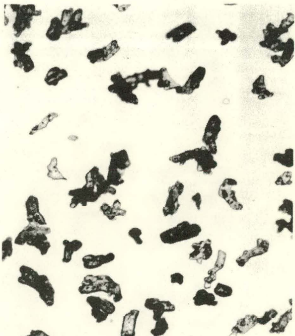
Sample Size 1.0 grams TATB Retained by 20 µm Sieve
