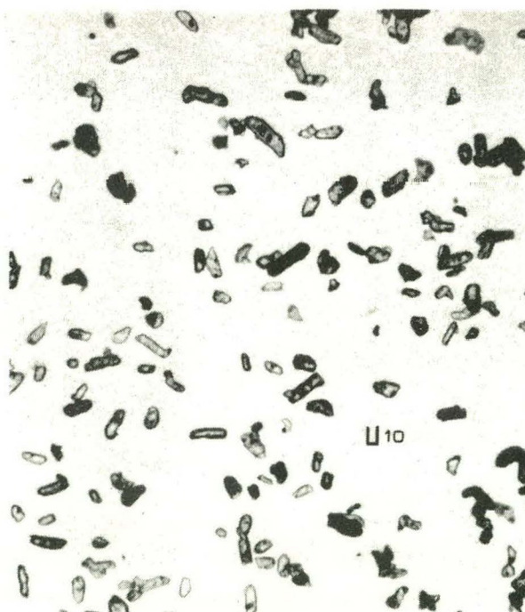
TATB Retained by 10 \mu\text{m} Sieve
