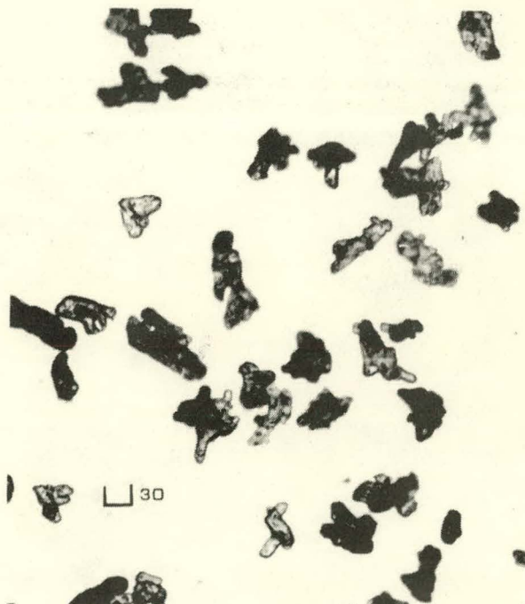
TATB Retained by 30 \mu\text{m} Sieve
