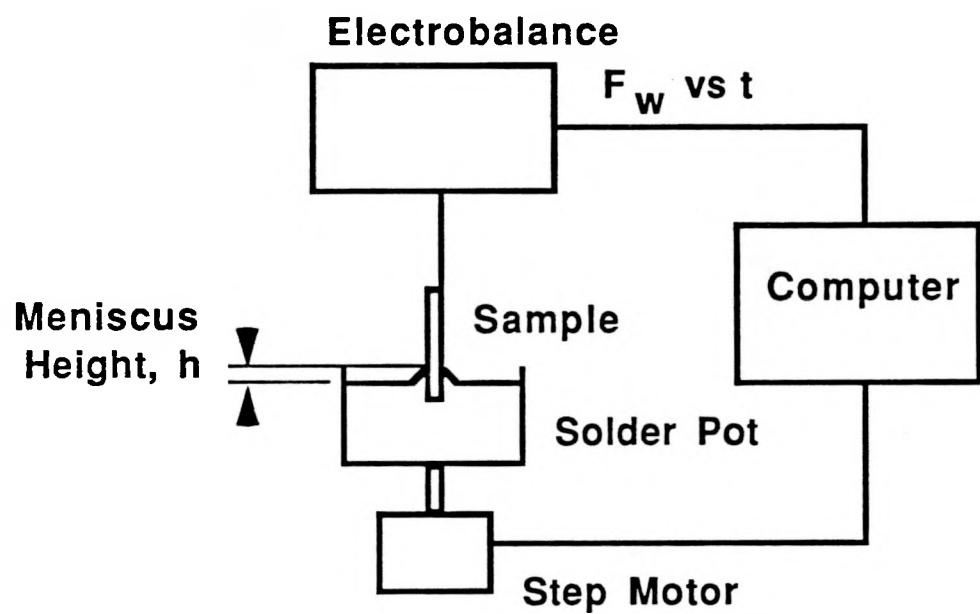
Figure 1. Schematic of the Sandia-designed Solder Wettability Test System
