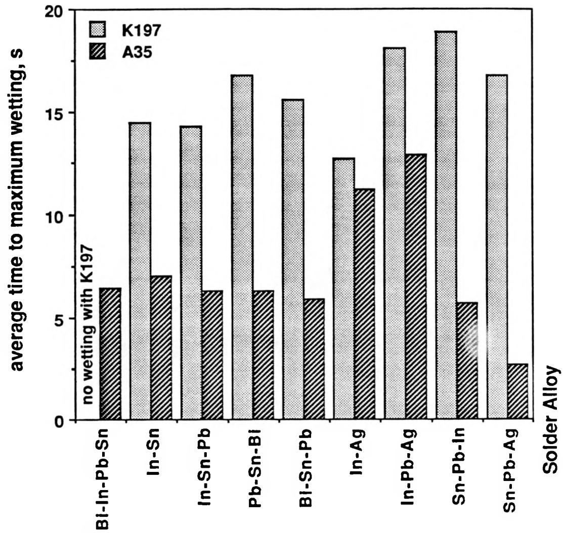
Figure 8. Average time to maximum wetting as a function of solder alloy and flux for Sn-Ni plated aluminum alloy wetting substrates.
