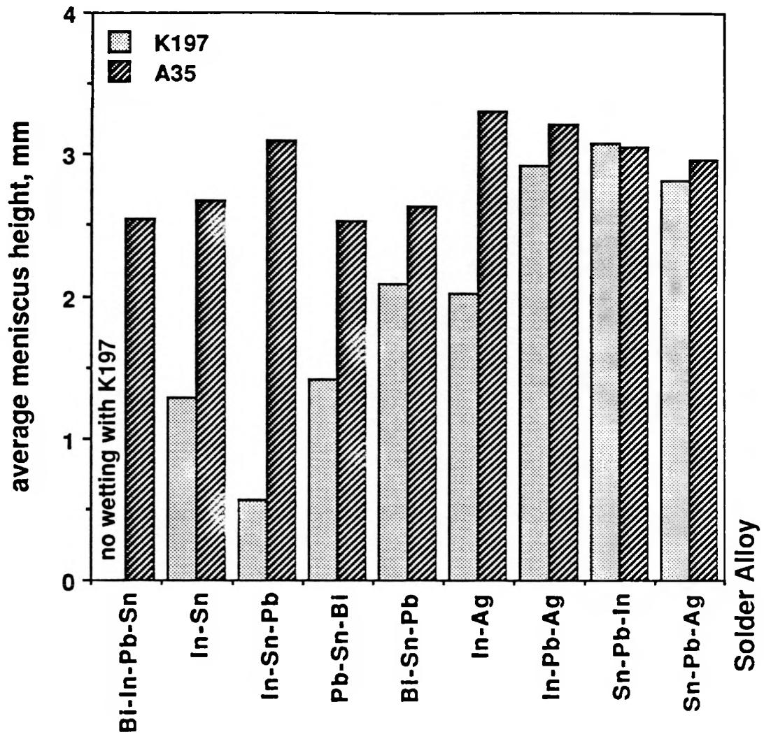
Figure 4. Average meniscus height as a function of solder alloy and flux for Sn-Ni plated aluminum alloy wetting substrates.
