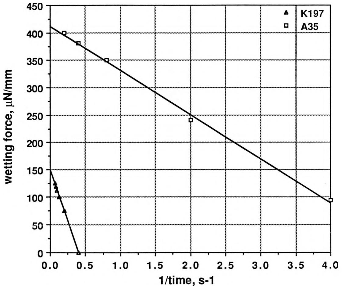
Figure 9. Wetting force as a function of  $\text{time}^{-1}$  for the K197 and A35 RMA fluxes at  $150^\circ\text{C}$  with the 40In-40Sn-20Pb solder alloy.
