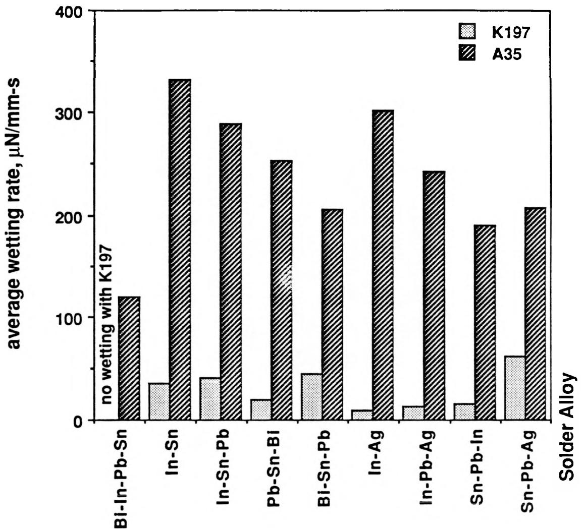
Figure 6. Average wetting rate as a function of solder alloy and flux for Sn-Ni plated aluminum alloy wetting substrates.
