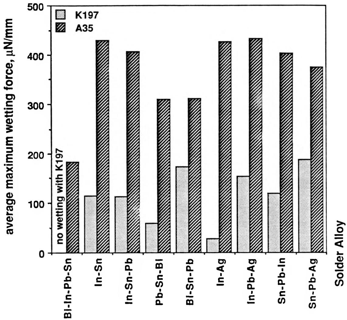
Figure 5. Average maximum wetting force as a function of solder alloy and flux for Sn-Ni plated aluminum alloy wetting substrates.
