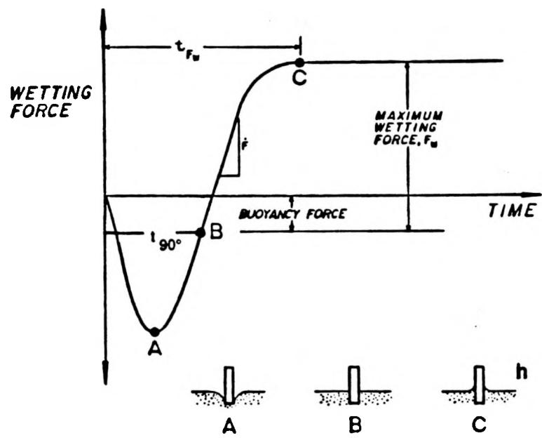
Figure 3. Typical wetting curve of force versus time measured by the wetting balance technique.
