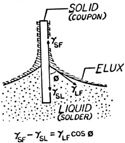
Figure 2. Schematic of the liquid solder, base metal, and flux surface tension equilibrium conditions for wetting of a vertical plate.
