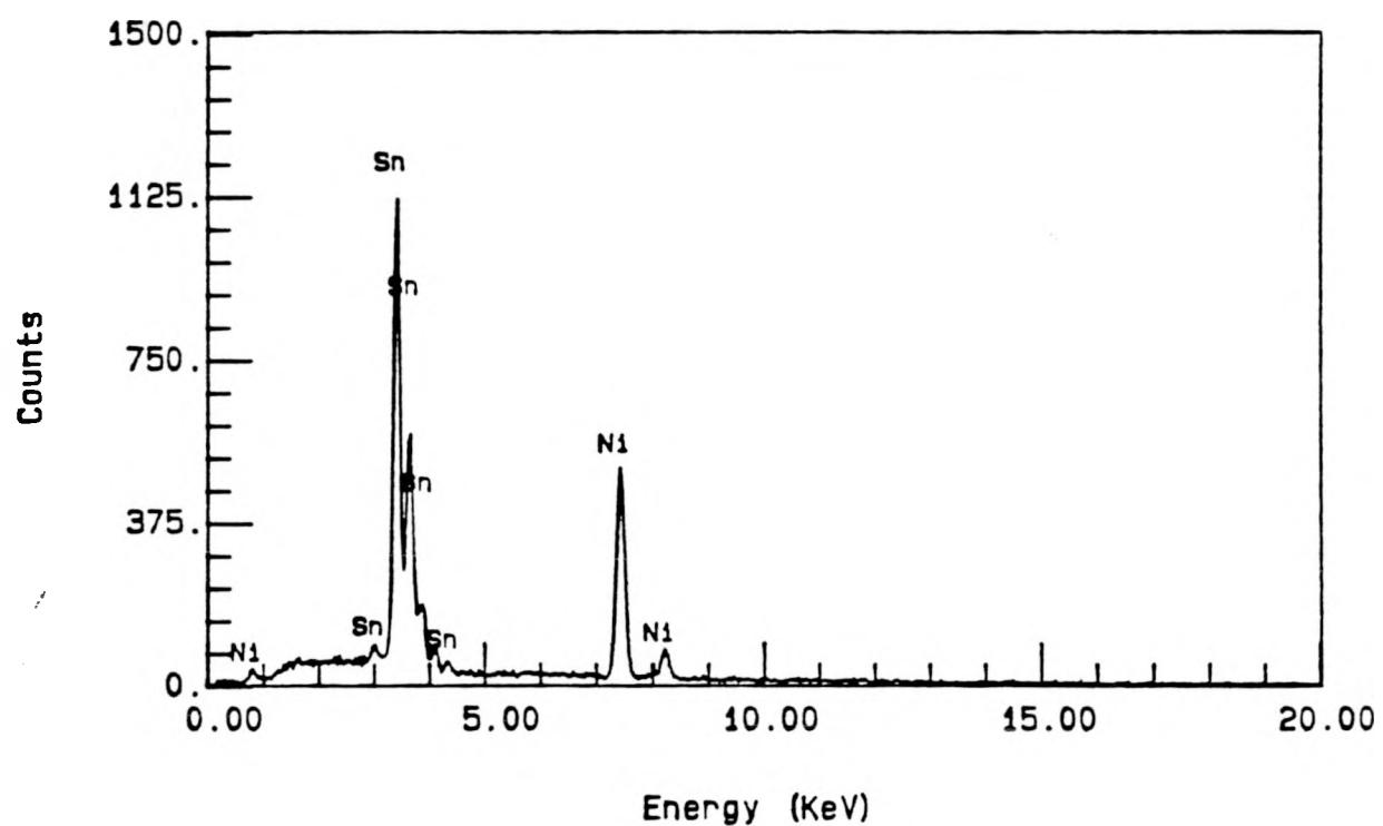
Figure 11. Energy dispersive spectrometry spectra of the Ni-Sn reaction layer between a 40In-40Sn-20Pb solder alloy and a plated Ni interface.
