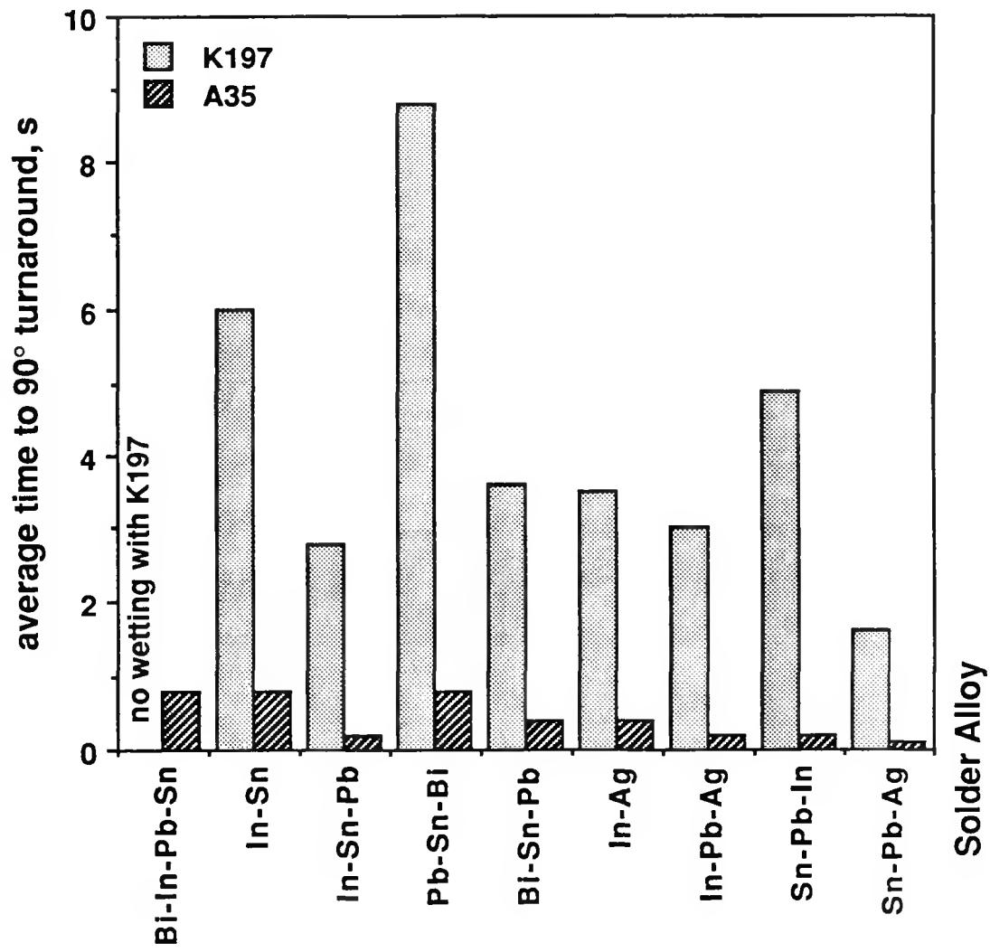
Figure 7. Average time to 90° turnaround as a function of solder alloy and flux for Sn-Ni plated aluminum alloy wetting substrates.
