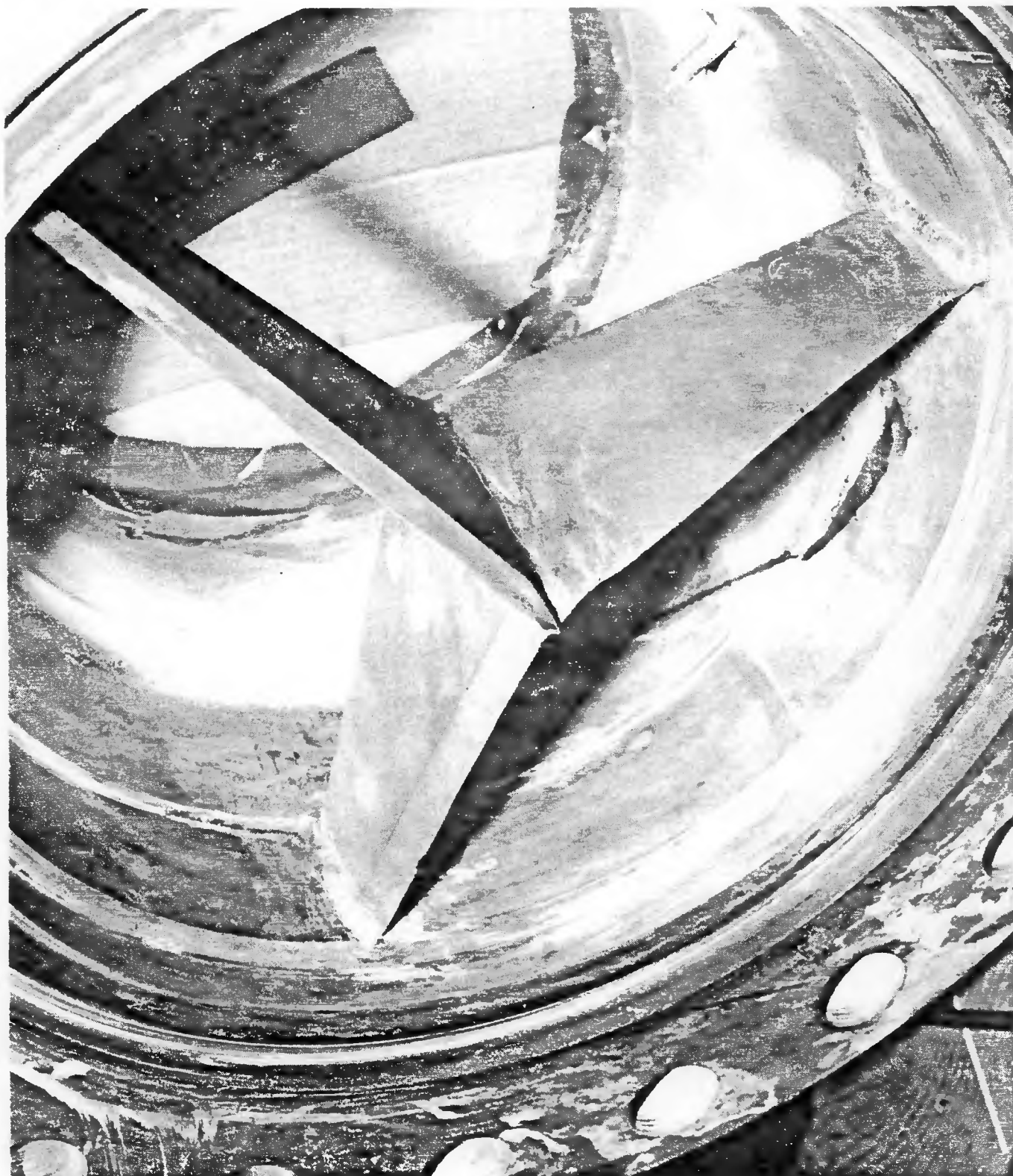
Figure VI-1. RUPTURE DISC BLADES AFTER TEST A-6
