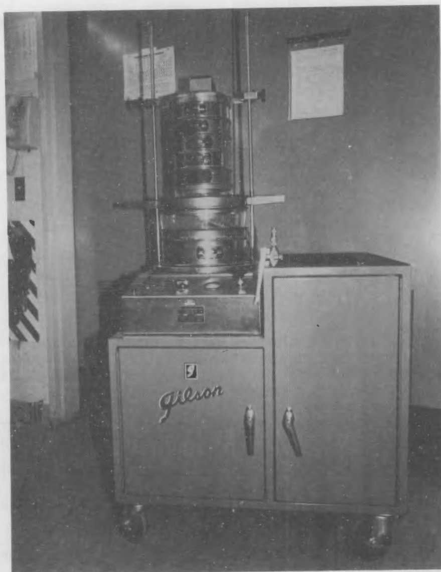
FIGURE 12. Gilson Wet Sieve Shaker Used for Tailings Particle Size Distribution Studies
