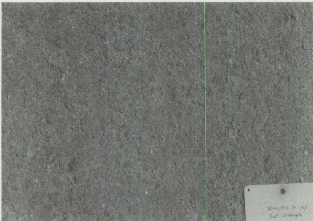
FIGURE 15. Test Plot Surface Stabilized with Wallpol 40-133 After 11 Months of Weathering (minor amount of surface erosion)
