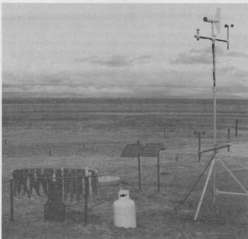
FIGURE 13. Weather Station Installed at Field Test
