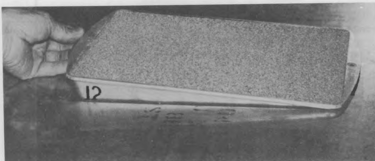
FIGURE 4. Sample Being Inserted in Cutout Floor Section of Wind Tunnel
