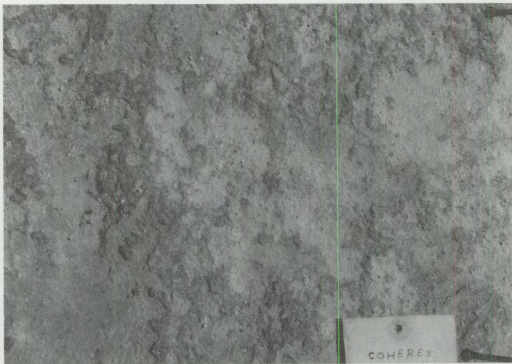
FIGURE 16. Test Plot Surface Stabilized with Coherex After 11 Months of Weathering (severe surface erosion)
